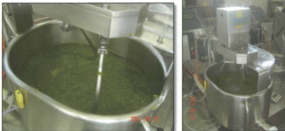
Figure 4.4. Ethanolic extraction of carotenoids
