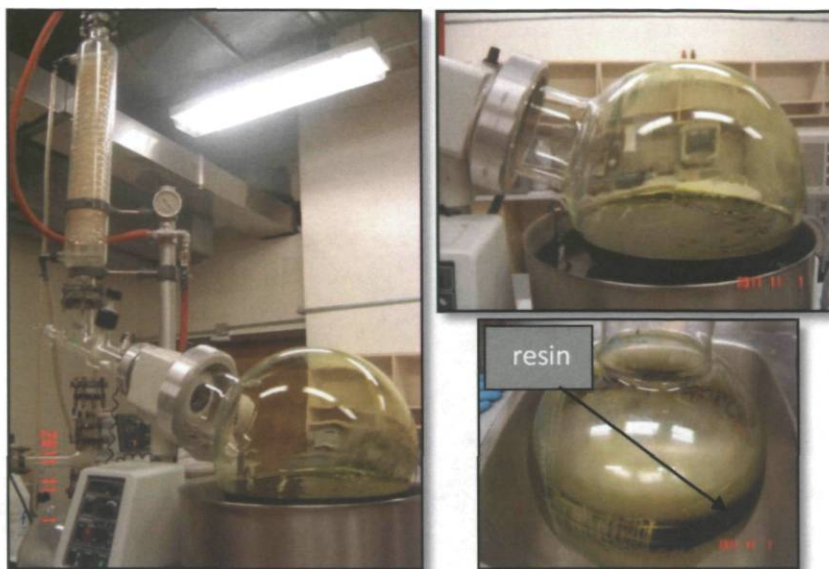
Figure 4.6. Evaporation of ethanol
