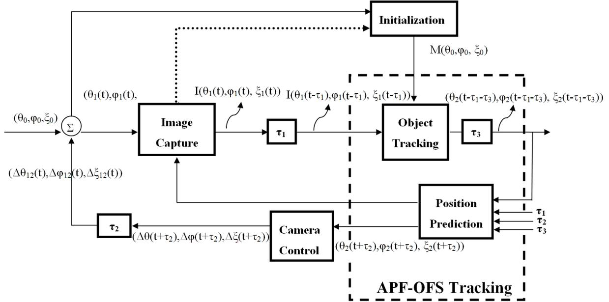
Figure 3.1. The system architecture and servo control model.  $(\theta_0, \varphi_0)$  : initial pan-tilt angles,  $\xi_0$ : initial zoom value,  $(\Delta\theta_{12}(t), \Delta\varphi_{12}(t), \Delta\xi_{12}(t))$  means  $(\theta_1 - \theta_2, \varphi_1 - \varphi_2, \xi_1 - \xi_2)$ ,  $M(\theta_0, \varphi_0, \xi_0)$ : target model,  $I(\theta(t), \varphi(t), \xi(t))$ : captured image at  $(\theta(t), \varphi(t), \xi(t))$ ,  $\Sigma$ : sum of inputs.
