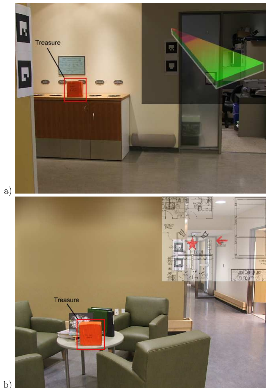
Figure 6.1: Examples of the mediated-reality tools, as perceived by the participant. a) The locator tool acts like a compass pointing to the treasure. In this example, the user needs to walk forwards and to the left to reach the treasure, resulting in a NW orientation of the locator. b) The minimap tool represents the position and orientation of the wheelchair as an arrow in the map, while the treasure is depicted as a star. In both examples, the “treasure” label was not seen by the user; it has been added simply to highlight the location of the treasure within these images.
