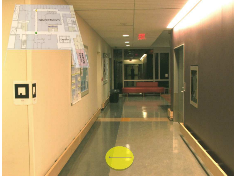
Figure 4.2: An example of what the user sees through the mediated reality display. A virtual compass (bottom-middle) and a virtual map of the environment (top-left) have been added to the real world using mediated reality.
