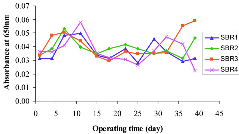
Figure C.4 Profile of effluent turbidity over the acclimation period.
