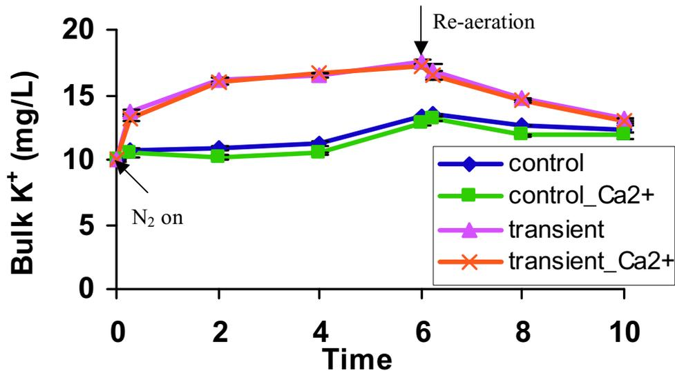
Figure 4.17 Changes of  $K^+$  under the addition of  $CaCl_2$ : Regardless of extra  $Ca^{2+}$ , the samples from both transient reactors had a higher level of  $K^+$  than those from control reactors under DO limitation. The error bars are +/- one standard deviation of bulk  $[K^+]$  measurements.
