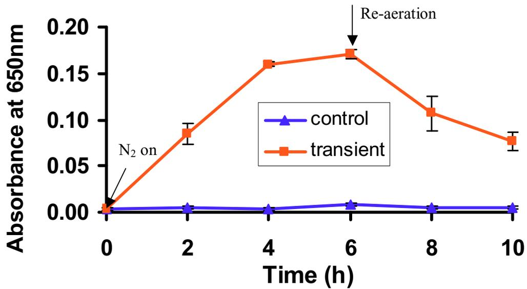
Figure 4.1 Typical turbidity changes under the DO transients: From  $t = 2$  to 6 hours of low DO, turbidity in the transient supernatants was significantly higher than that in the control ones ( $p = 2.9 \times 10^{-4}$ ). The error bars are +/- one standard deviation of turbidity measurements.
