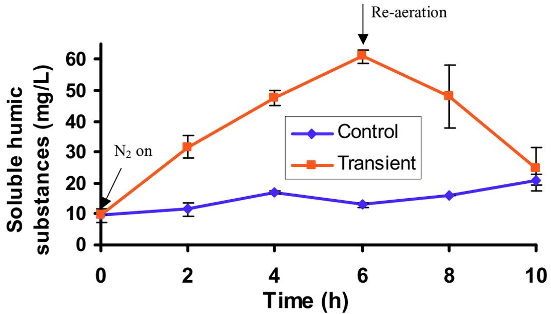
Figure 4.7 Typical changes in soluble humic substances under DO transients: From  $t = 2$  to 6 hours, soluble humic substances in the transient samples were significantly higher than those in the control samples ( $p = 6.3 \times 10^{-5}$ ). The error bars are +/- one standard deviation of bulk proteins.
