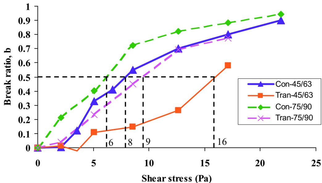
Figure 4.30 Shear strength of bioflocs from the control reactor (SBR2) and the transient reactor (SBR4): for both samples within 45-63  $\mu\text{m}$  and 75-90  $\mu\text{m}$ , bioflocs in SBR4 were stronger than those in SBR2.
