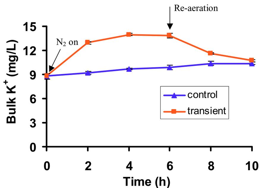
Figure 4.10 Typical changes in bulk  $K^+$  under DO transients: From  $t = 2$  to 6 hours, the transient samples had a higher concentration of bulk  $K^+$  than the control samples ( $p = 3.5 \times 10^{-7}$ ). The error bars are +/- one standard deviation of bulk  $[K^+]$  measurements.
