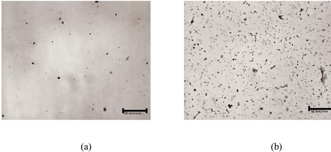
Figure 4.2 Microscopic observation of supernatant (stage I): (a) control; (b) transient. The images were taken by Axiovert 200, inverted microscope. The bar represents 50  $\mu\text{m}$ .
