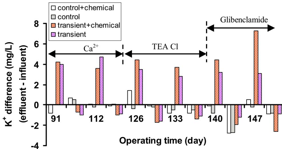
Figure 4.33 Changes in extracellular  $K^+$  after adding the selected chemicals: adding extra  $Ca^{2+}$ , TEA chloride and glibenclamide failed to prevent the release of  $K^+$  under DO limitation. Transient days are labelled on x-axis. The error bars are  $\pm$  one standard deviation.
