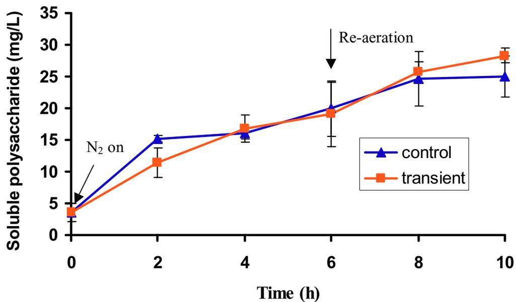
Figure 4.9 Changes in soluble polysaccharides under DO transients: There were no significant difference between the control and transient samples from  $t = 2$  to 6 hours ( $p = 0.43$ ). The error bars represent  $\pm$  one standard deviation of bulk polysaccharides.
