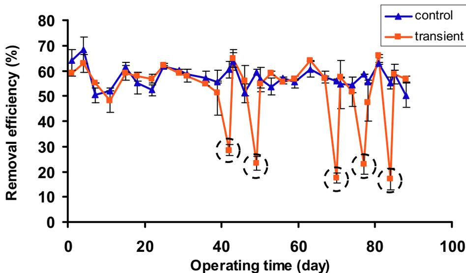
Figure 4.21 Removal of SCOD under DO transients: SCOD removal in the control reactors remains stable throughout the experiments. In the transient reactors, removal of SCOD significantly decreased from approximately 60% to less than 30% ( $p = 6.2 \times 10^{-6}$ ). Transient days are days 42, 49, 70, 77 and 84, as marked by cycles. Each data point represents the mean value with  $\pm$  one standard deviation.
