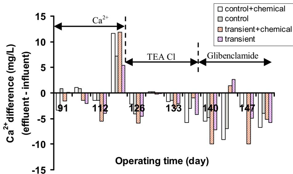
Figure 4.34 Changes in extracellular  $Ca^{2+}$  after adding the selected chemicals: adding extra  $Ca^{2+}$ , TEA chloride and glibenclamide failed to prevent the reduction of  $Ca^{2+}$  under DO limitation. Transient days are labelled on x-axis. The error bars are  $\pm$  standard deviation.
