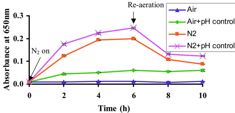
Figure E.2 Turbidity changes under the DO stress with pH control: Both DO-stressed reactor had the higher turbidity than the control ones. Reactor “N<sub>2</sub> + pH control” has the highest turbidity.
