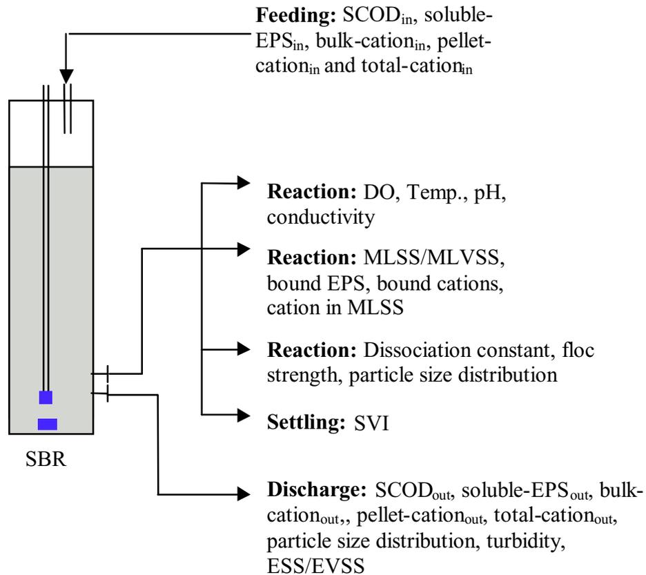
Figure 3.7 Data collection within an operating cycle from a SBR
