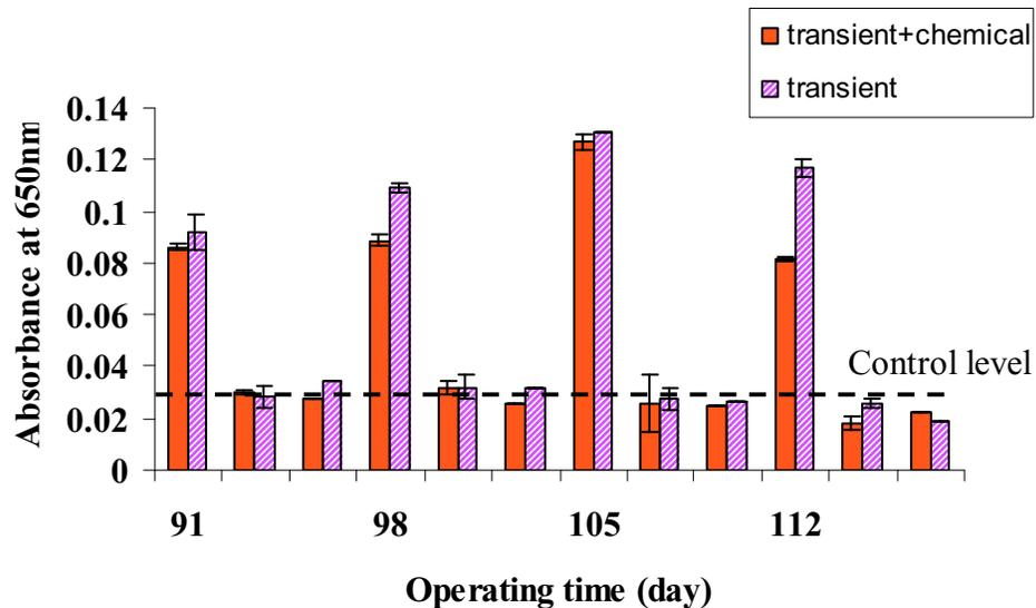
Figure 4.31 Changes of effluent turbidity upon DO variations from days 91 to 116. On transient days (labelled on x-axis), the addition of  $\text{Ca}^{2+}$  into the transient reactor partially alleviated the increasing turbidity, as shown by the lower turbidity than those in the transient reactor without  $\text{Ca}^{2+}$  ( $p = 0.012$ ). The error bars are +/- one standard deviation.
