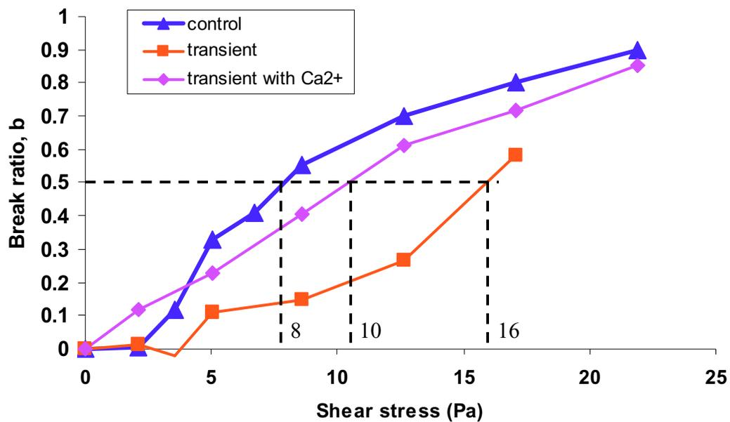
Figure 4.35 Distribution of shear strength of control reactor SBR2, transient reactors SBR3 (enriched with  $\text{Ca}^{2+}$ ) and SBR4 for the bioflocs of 45-63  $\mu\text{m}$ . Addition of  $\text{Ca}^{2+}$  reduced the shear strength of DO-stressed bioflocs.
