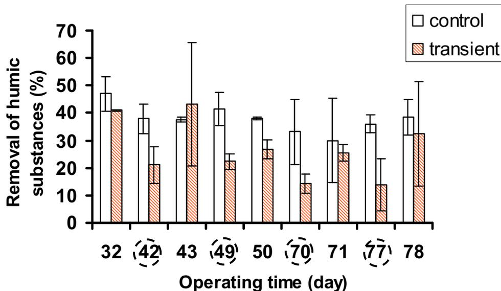
Figure 4.25 Removal of humic substances under DO transients: a decreasing removal efficiency of humic substance was shown in the transient SBRs ( $p = 3.7 \times 10^{-4}$ ) on transient days 42, 49, 70 and 77 (as marked by cycles). The error bars are  $\pm$  one standard deviation of the measurements.
