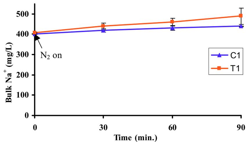
Figure D.3.1 Changes in bulk  $Na^+$  in a typical *E. coli* test: there was insignificant difference between the control and transient data ( $p = 0.09$ ). The error bars are  $\pm$  one standard deviation of the measurements.
