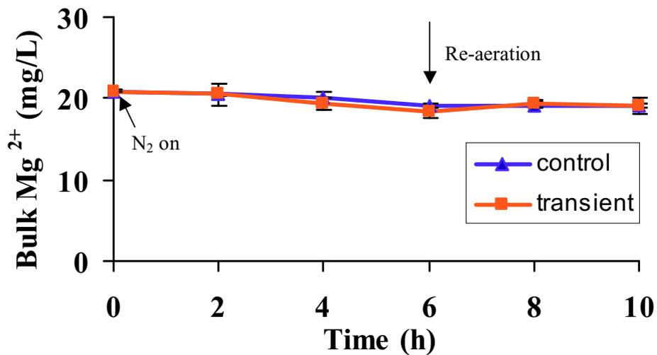
Figure D.1.2 Changes in bulk  $Mg^{2+}$  in a typical DO test: There was insignificant difference between the control and transient data ( $p = 0.20$ ). The error bars are +/- one standard deviation of the measurements.
