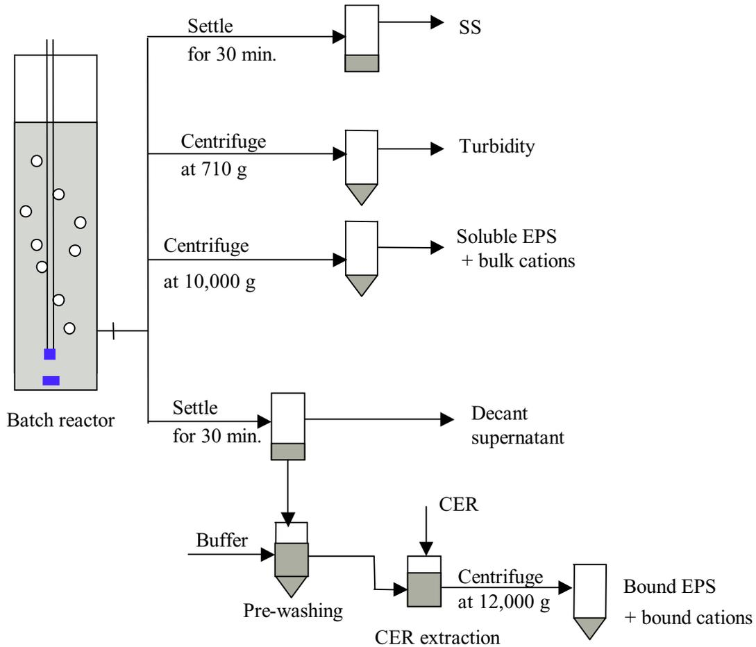
Figure 3.4 A schematic diagram of sample treatment in batch experiments
