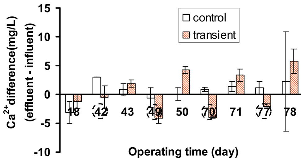
Figure 4.27 Changes in extracellular  $\text{Ca}^{2+}$  under DO transient: each column represents the  $\text{Ca}^{2+}$  difference between the treated effluents and untreated influents.  $\text{O}_2$  stress caused a reduction of  $\text{Ca}^{2+}$  in treated effluents ( $p=2.0 \times 10^{-3}$ ), as shown on transient days 42, 49, 70 and 77. The error bars are +/- one standard deviation of the measurements.
