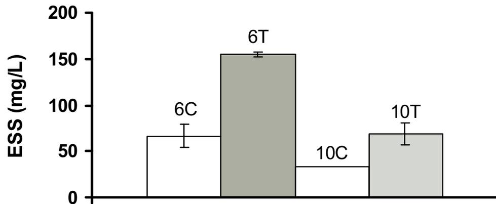
Figure 4.3 Typical changes in SS concentrations under DO transients: “6C” is the control sample at  $t = 6$  hours ( $DO > 5$  mg/L); “6T” is the transient sample at  $t = 6$  hours ( $DO < 0.5$  mg/L); “10C” is the control sample at  $t = 10$  hours ( $DO > 5$  mg/L); “10T” is the transient sample at  $t = 10$  hours ( $DO > 5$  mg/L). The error bars represent  $\pm$  one standard deviation of SS measurements.
