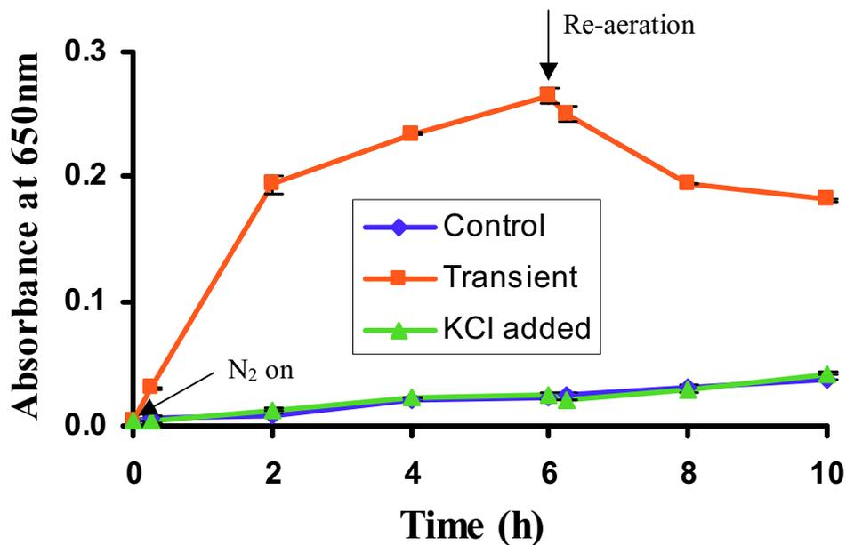
Figure 4.13 Turbidity changes under the addition of KCl: The samples exposed to a DO limitation had the highest turbidity. There was insignificant difference between control samples and KCl-added samples ( $p = 0.18$ ). The error bars are +/- one standard deviation of turbidity measurements
