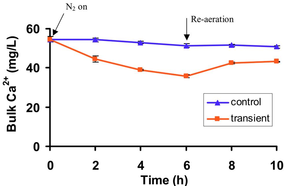
Figure 4.11 Changes of bulk Ca<sup>2+</sup> under DO transients: From t = 2 to 6 hours, the transient samples had a lower concentration of bulk Ca<sup>2+</sup> than the control samples ( $p = 3.9 \times 10^{-5}$ ). The error bars are +/- one standard deviation of bulk [Ca<sup>2+</sup>] measurements.
