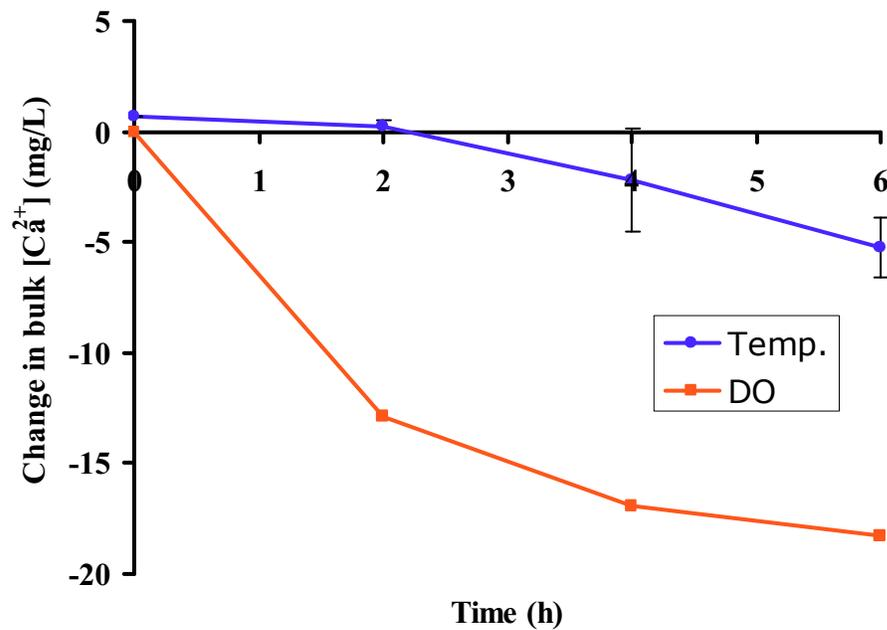
Figure G.3 Comparison of the changes in bulk  $Ca^{2+}$ : Changes in bulk  $Ca^{2+}$  under temperature upshift were lower than those under DO limitation over the experimental time.
