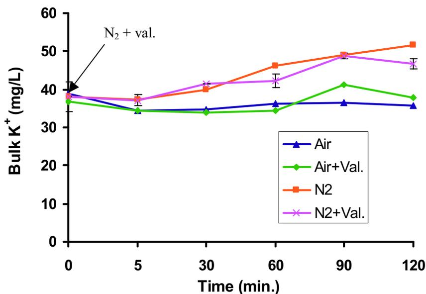
Figure 4.42 Changes in bulk  $K^+$  with the addition of valinomycin: In spite of adding valinomycin,  $O_2$  shortage caused increasing levels of bulk  $K^+$ . Valinomycin is denoted as “Val.” The error bars are the +/- one standard deviation of bulk  $K^+$ .
