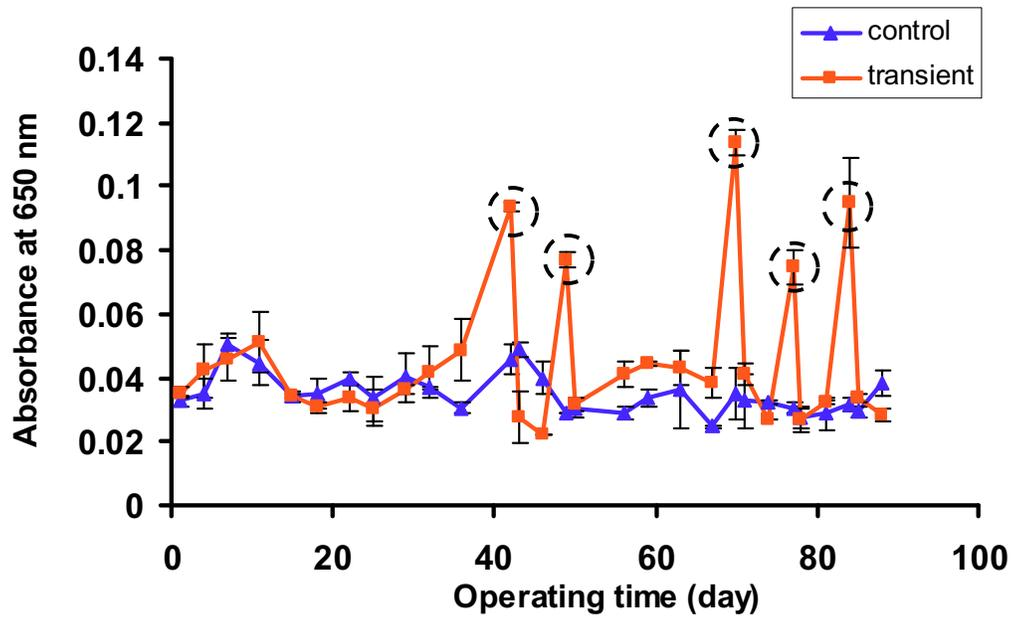
Figure 4.23 Changes in effluent turbidity under DO transients: transient turbidity (as marked by cycles) was significantly higher than in the control reactor on transient days 42, 49, 70, 77 and 84 ( $p = 9.4 \times 10^{-4}$ ). Each data point represents the mean value with  $\pm$  one standard deviation.
