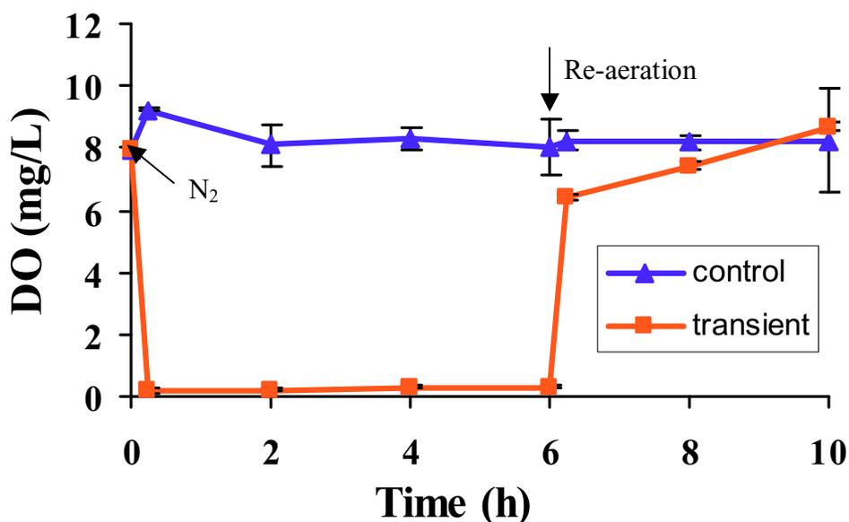
Figure 3.3 An example of DO profile in a typical batch experiment: DO level in the control reactor were kept around 8mg/L; DO levels in the transient reactors were below 0.5mg/L in the first 6 hours. The error bars are the +/- one standard deviation of DO measurements.
