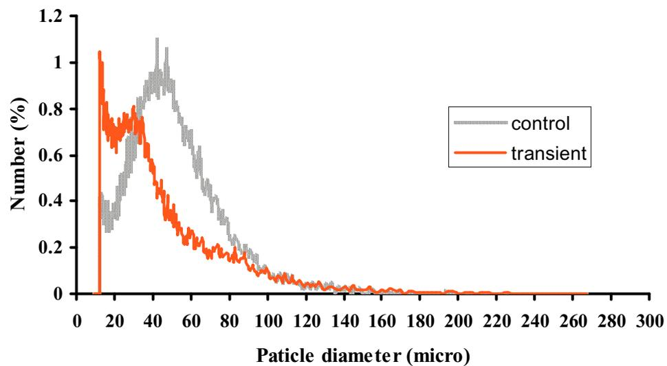
Figure 4.29 Particle size distribution of mixed liquor samples on day 98: The transient sample had a higher amount of small particles ( $< 20 \mu\text{m}$ ) than the control sample.
