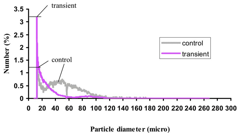
Figure 4.28 Effluent particle size distribution in treated effluents on day 98: The transient effluent had a higher amount of small particles ( $< 20 \mu\text{m}$ ) than the control effluent.
