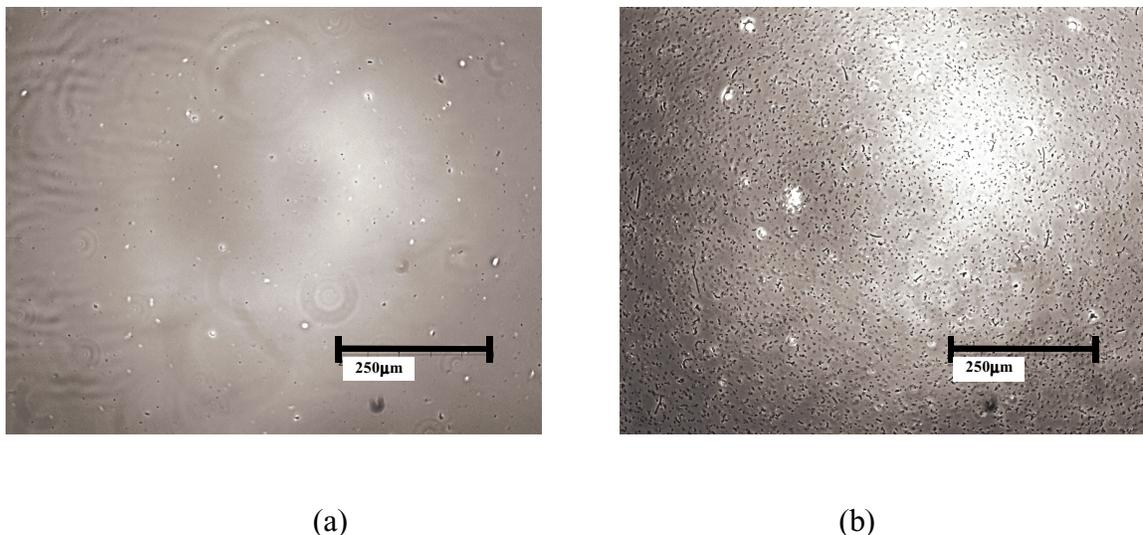
Figure 4.20 Microscopic observation of supernatant in trypsin test: (a) control; (b) transient. The image was taken 8 hours after the addition of trypsin by Axiovert 200, inverted microscope. The bar represents 250  $\mu\text{m}$
