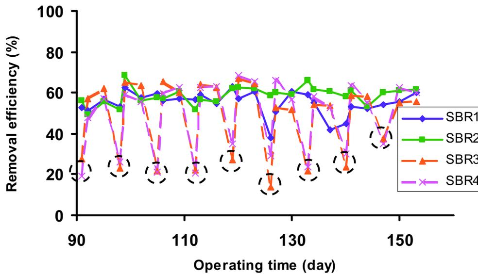
Figure 4.32 Removal of SCOD from days 91-156: In spite of the added chemicals, the removal of SCOD in the transient reactors declined under low DO (marked by cycles). Each data point represents the mean value with +/- one standard deviation.
