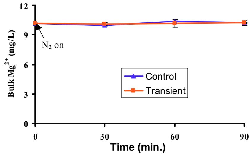
Figure D.3.2 Changes of bulk  $Mg^{2+}$  in a typical *E. coli* test: there was no significant difference between the control and transient data ( $p = 0.24$ ). The error bars are +/- one standard deviation of the measurements.
