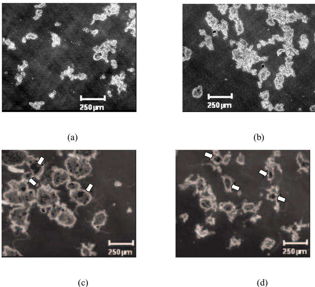
Figure 4.36 Microscopic observations of bioflocs on day 133: (a) Control (SBR2); (b) Transient (SBR4); (c) Control+  $\text{Ca}^{2+}$ /TEA chloride(SBR1); (d) Transient +  $\text{Ca}^{2+}$ /TEA chloride
