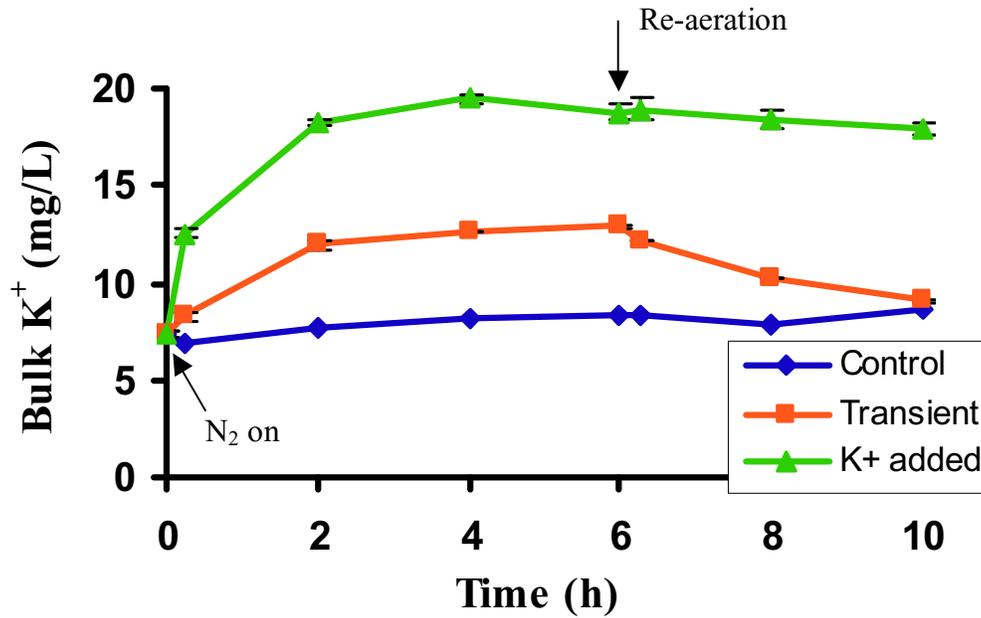
Figure 4.14  $K^+$  in the soluble solution under the addition of KCl: Addition of KCl caused the highest level of bulk  $K^+$ , higher than the  $K^+$  increment due to DO limitation. The error bars are  $\pm$  one standard deviation of bulk  $[K^+]$  measurements.
