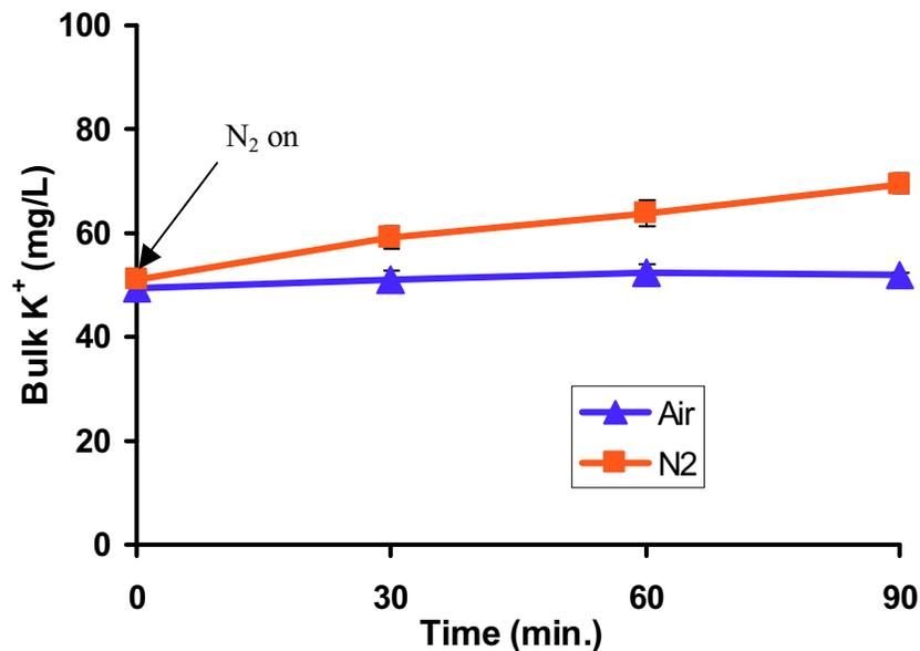
Figure 4.39 Changes of bulk  $K^+$  in *E. coli* cultures responding to  $O_2$  limitation: the stressed samples (denoted as “N2”) had higher concentrations of bulk  $K^+$  than the control samples ( $p = 0.002$ ). The error bars are +/- one standard deviation of the measurements.
