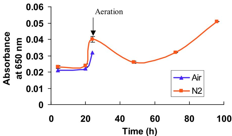
Figure A.1 Turbidity changes under DO variations: Only 5 min of N<sub>2</sub> purging was applied in the first 20 hours, there was insignificant difference between the control and transient samples; from the 20<sup>th</sup> to the 24<sup>th</sup> hours, 5 min of N<sub>2</sub> purging was applied every hour, transient samples showed a higher turbidity than the control sample. After re-aeration at the 24<sup>th</sup> hours, transient
