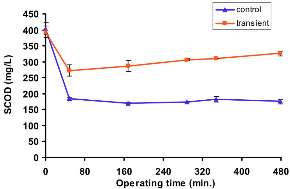
Figure 4.22 SCOD profile in an 8-hour operating cycle: transient reactors had a higher SCOD than control ones. Average transient SCOD increased by 13% from  $t = 160$  to 480 min. Each data point represents the mean value with  $\pm$  one standard deviation.
