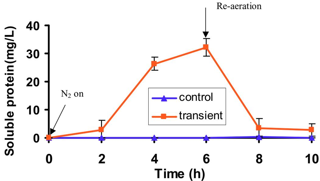
Figure 4.5 Typical changes in soluble proteins under DO transients: From  $t = 2$  to 6 hours, soluble proteins in the transient samples were significantly higher than those in the control samples ( $p = 2.3 \times 10^{-3}$ ). The error bars are +/- one standard deviation of bulk proteins.
