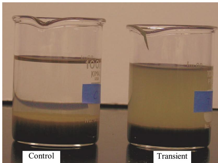
Figure 4.4 Image of supernatants at  $t = 6$  hours: The transient sample had more cloudy supernatants than the control sample
