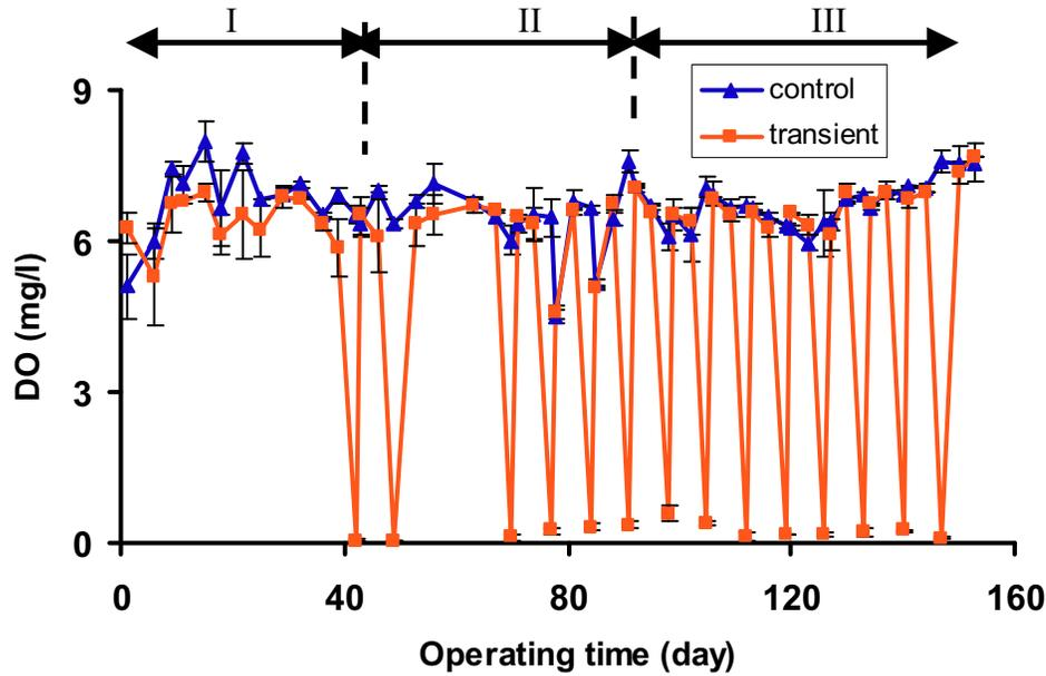
Figure 3.6 Dissolved oxygen (DO) in SBRs in the periods of acclimation (I), identifying deflocculation (II) and testing strategy (III). Control curve was the average DO values of SBR1 and SBR2 whereas transient curve was the average DO values of SBR3 and SBR4. Each data point represents the mean value with  $\pm$  one standard deviation.
