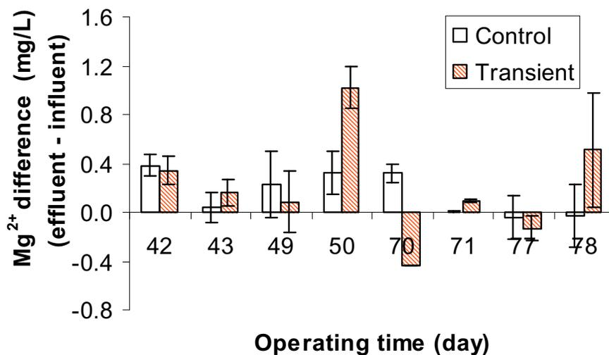
Figure D.2.2 Changes of  $Mg^{2+}$  difference upon DO variations: Transient days are 42, 49, 70 and 77. There was insignificant difference between the control and transient samples ( $p = 0.22$ ). The error bars are  $\pm$  one standard deviation of the measurements.
