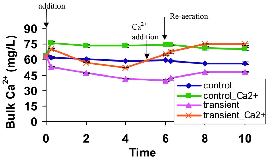
Figure 4.18 Changes of  $\text{Ca}^{2+}$  under the addition of  $\text{CaCl}_2$ : Extra  $\text{Ca}^{2+}$  was introduced at  $t = 0$  and  $t = 5$  hours. In spite of adding  $\text{Ca}^{2+}$ , the samples from transient reactors had declining levels of bulk  $\text{Ca}^{2+}$  under DO limitation. The error bars are  $\pm$  one standard deviation of bulk  $[\text{Ca}^{2+}]$  measurements.
