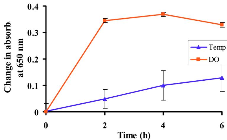
Figure G.1 Comparison of turbidity changes: DO transients caused much higher turbidity in the first 2 hours, probably due to the sharp decline in the DO levels.
