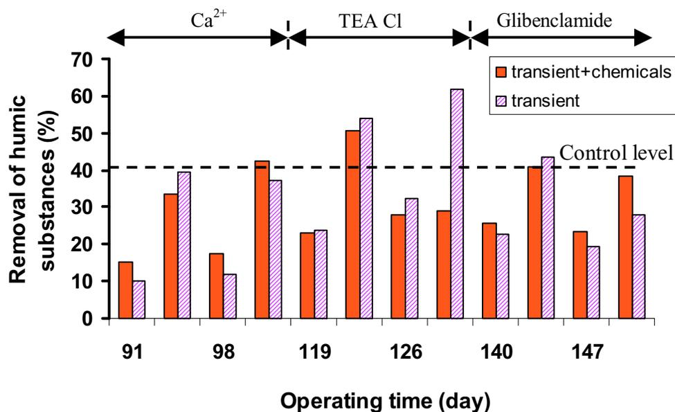
Figure 4.37 Removal of humic substances from days 91-150: Compared to the transient reactor without the added chemicals, the addition of  $\text{Ca}^{2+}$  and glibenclamide into the transient reactors appeared to enhance the removal efficiency on transient days 91, 98, 140 and 147, as shown by the higher columns than the ones without the chemicals.
