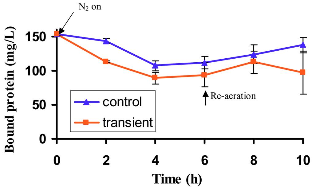
Figure 4.6 Typical changes in bound proteins under DO transients: From  $t = 2$  to 6 hours, the transient samples had a lower concentration of bound proteins than the control samples ( $p = 0.035$ ). The error bars are  $\pm$  one standard deviation of bound protein measurements.
