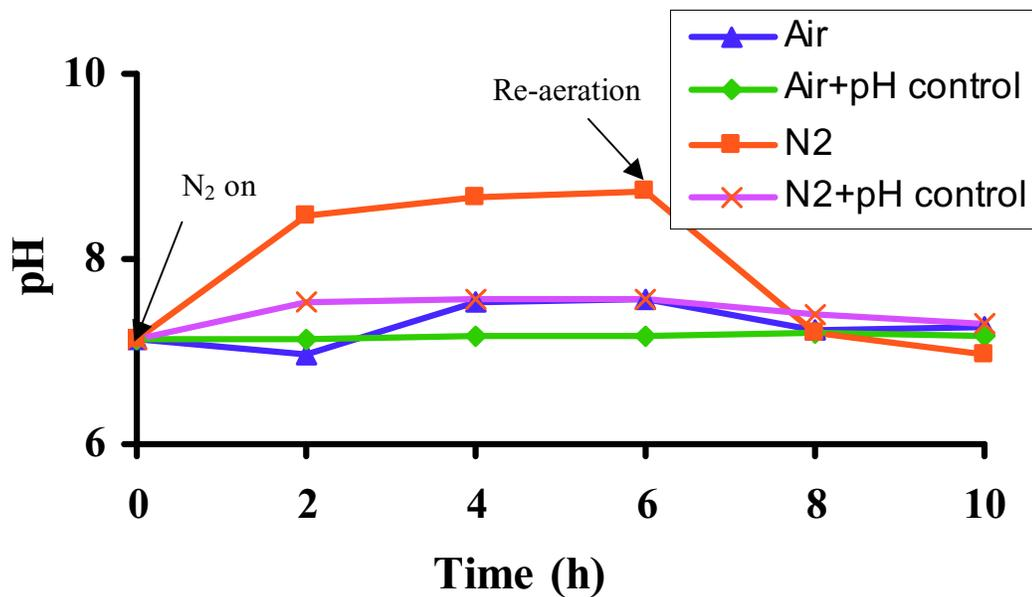
Figure E.1 pH profile in a typical DO test with pH control.
