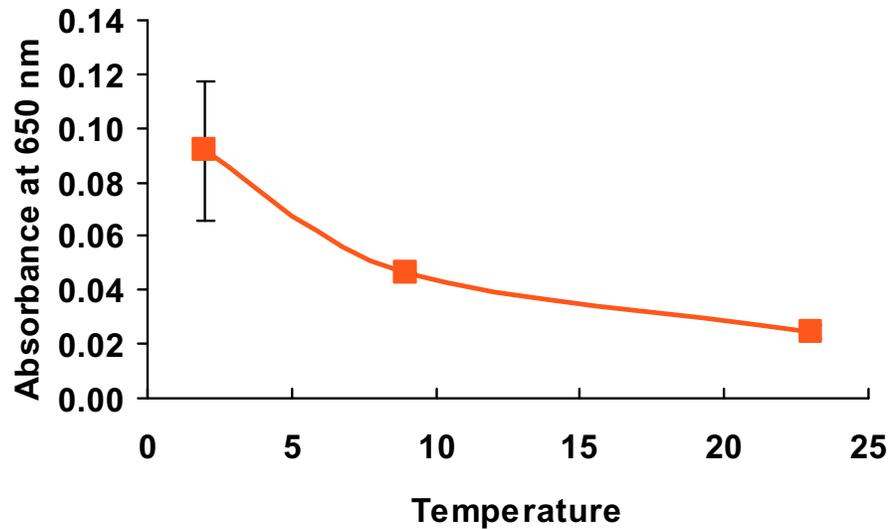
Figure A.2 Turbidity changes under temperature downshifts: Turbidity increased significantly when the temperature dropped below 4°C. The error bars are +/- one standard deviation of the measurements.
