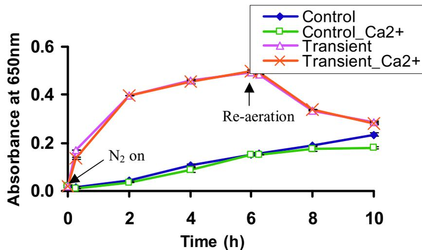
Figure 4.16 Changes of turbidity under the addition of  $\text{CaCl}_2$ : The samples exposed to DO limitation had the highest turbidity. Regardless of extra  $\text{Ca}^{2+}$ , there was no significant difference between turbidity in the transient reactors ( $p = 0.36$ ). The error bars are  $\pm$  one standard deviation of turbidity measurements.
