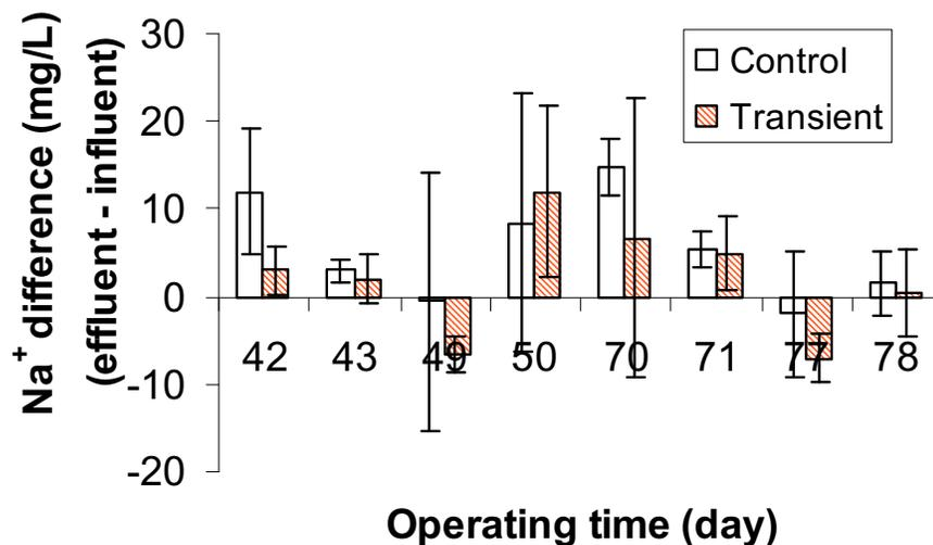
Figure D.2.1 Changes of  $Na^+$  difference upon DO variations: Transient days are 42, 49, 70 and 77. There was insignificant difference between the control and transient samples ( $p = 0.17$ ). The error bars are +/- one standard deviation of the measurements.
