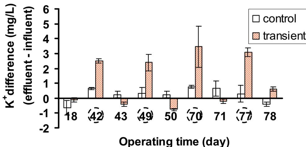
Figure 4.26 Changes in extracellular  $K^+$  under DO transients: each column represents  $K^+$  difference between the treated effluents and untreated influents. More  $K^+$  were released into effluents on transient days 42, 49, 70 and 77 ( $p = 2.1 \times 10^{-3}$ ). The error bars are  $\pm$  one standard deviation of the measurements.
