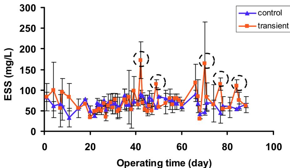
Figure 4.24 Effect of DO transients on ESS: Despite relatively high variations in the measurements, ESS concentrations in the transient reactors (as marked by cycles) were significantly higher than those in the control reactors on transient days 42, 49, 70, 77 and 84 ( $p = 2.6 \times 10^{-3}$ ). Each data point represents the mean value with  $\pm$  one standard deviation.
