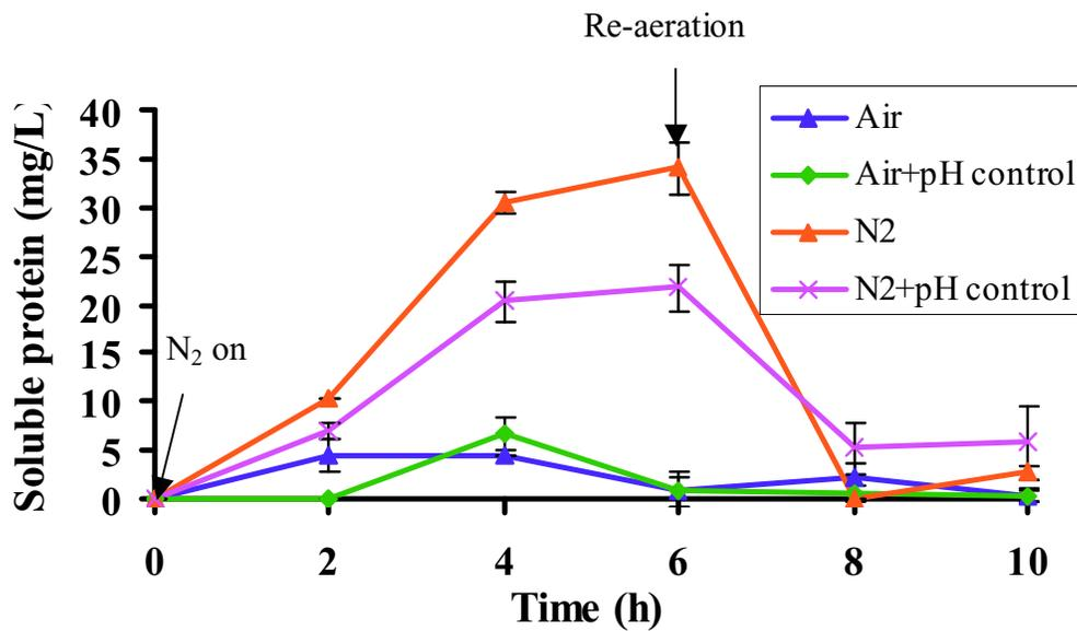
Figure E.3 Changes in soluble proteins in a typical DO test with pH control. The error bars are +/- one standard deviation of the measurements.
