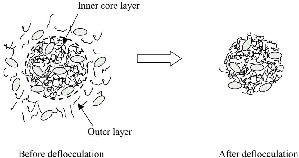
Figure 5.1 A schematic diagram of the change in bioflocs' structure under deflocculation (modified from Liao et al. (2002)).
