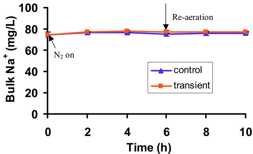
Figure D.1.1 Changes in bulk  $\text{Na}^+$  in a typical DO test: There was insignificant difference between the control and transient data ( $p = 0.12$ ).
