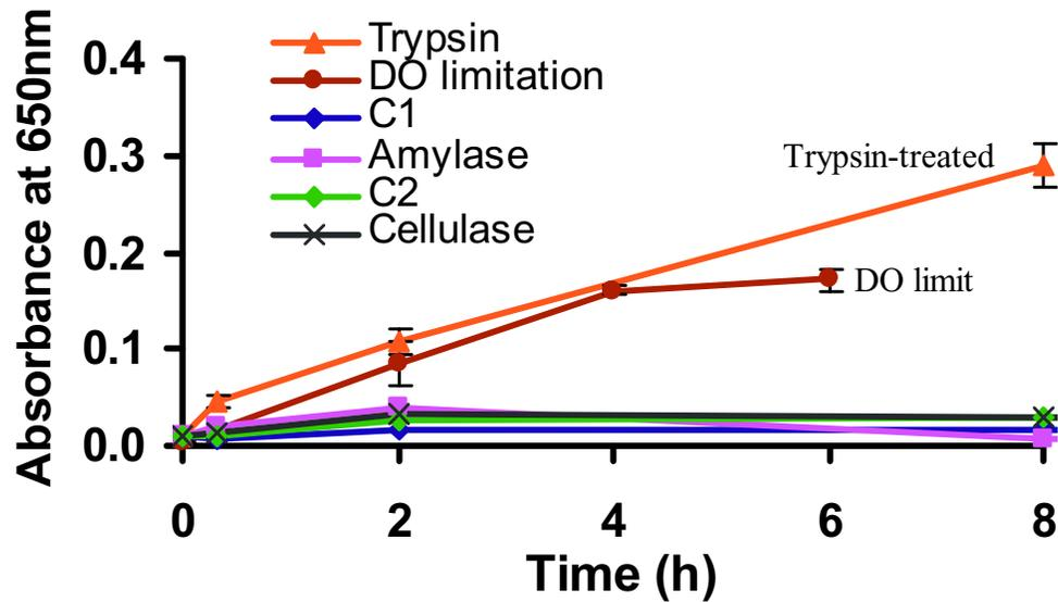
Figure 4.19 Turbidity changes in enzyme tests: Operating temperatures for trypsin and cellulase were 37°C, for amylase was 25°C. Two reference samples were prepared at 25°C (C1) and 37°C (C2), respectively. The trypsin-treated samples had the highest turbidity increment over the time. The error bars represent +/- one standard deviation of turbidity measurements.
