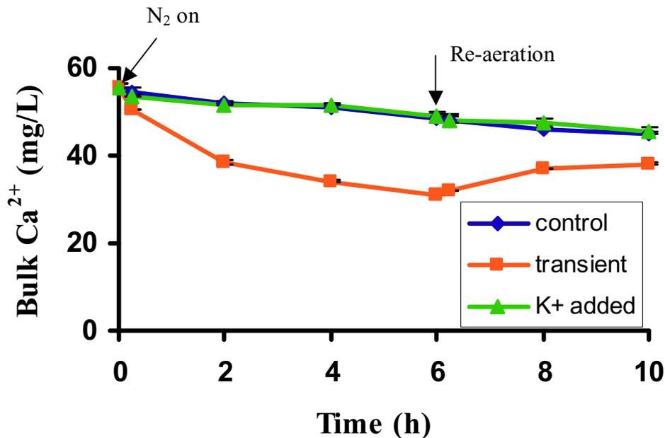
Figure 4.15 Ca<sup>2+</sup> in the soluble solution under the addition of KCl: The samples exposed to DO limitation had the declining levels of bulk Ca<sup>2+</sup>. There was insignificant difference between control samples and KCl-added samples ( $p = 0.29$ ). The error bars are +/- one standard deviation of bulk [Ca<sup>2+</sup>] measurements.
