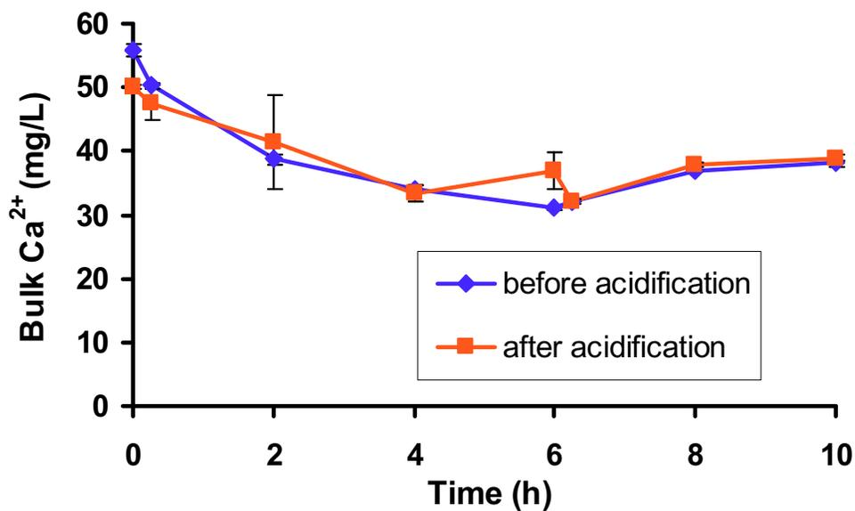
Figure 4.12 Changes of  $\text{Ca}^{2+}$  under acidification: There was no significant difference between the samples before and after acidification ( $p = 0.59$ ). The error bars are +/- one standard deviation of  $[\text{Ca}^{2+}]$  measurements.
