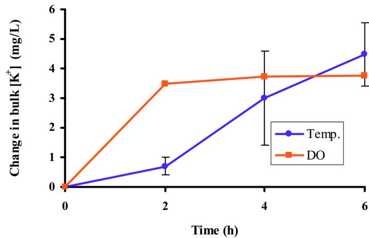
Figure G.2 Comparison of changes in bulk  $K^+$ : In the first 2 hours, the increase in bulk  $K^+$  under DO limitation was much higher than that under temperature upshift.
