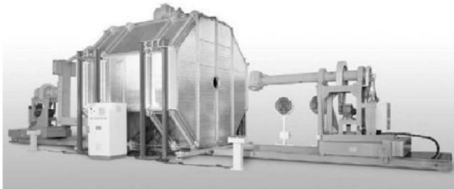
Figure 2-3: Two-station shuttle machine [31]
