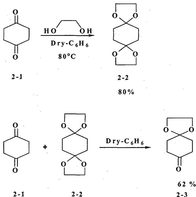
**Scheme 2-4.** Synthesis of **2-3** using a Dean Stark trap for azeotropic removal of water
