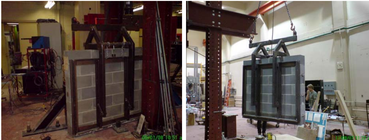
Figure 3.16: The Steel Frame Manufactured to Lift Walls
