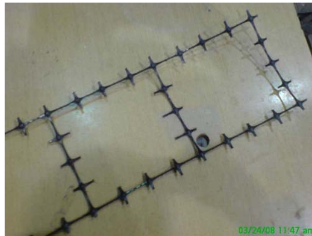
Figure 3.11: Geogrid Bed Joint Reinforcement (Ladder Shape) used in Wall-E(L)
