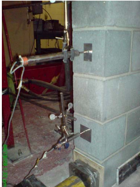
Figure 3.19: Locations of LSCs on the Left Side of the Wall
