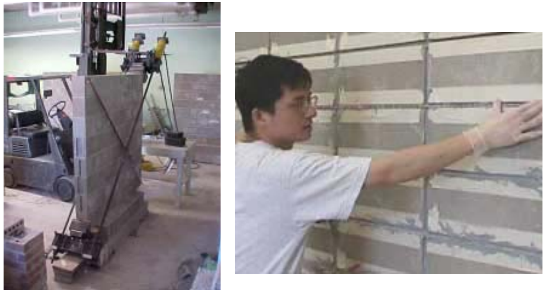
Figure 2.9: Test Setup (left) and Installation of GFRP Bars (right) [Tumialan et al. 2001]
