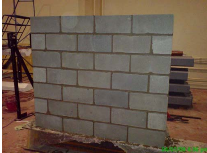
Figure 3.7: The Typical Control Wall “Wall-C”
