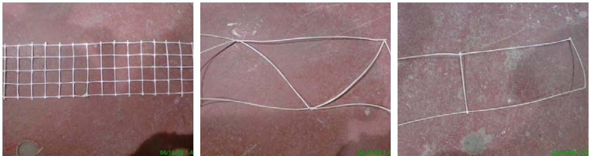
Figure 3.4: GFRP Bed Joint Reinforcement (Grid, Truss, and Ladder Shapes)
