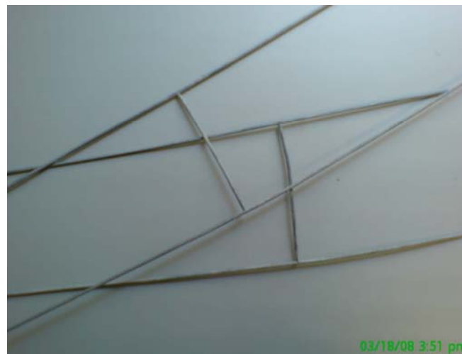
Figure 3.2: Steel Bed Joint Reinforcement (Ladder shape)
