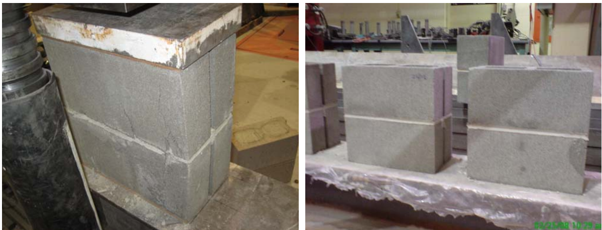
Figure 3.1: Compression Test (left) and Two-High UngROUTED Face Shell Bedded Prisms (right)
