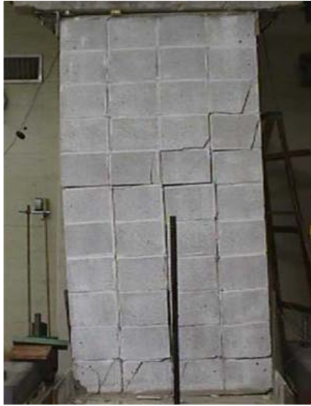
Figure 2.8: Ultimate State of the Wall Retrofitted with Horizontal GFRP Rods [Li et al. 2001]
