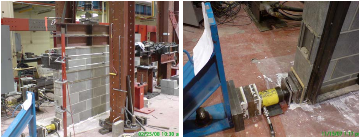
Figure 3.17: Steel Rods, I-Beam (left) and the Hydraulic Pump (right)
