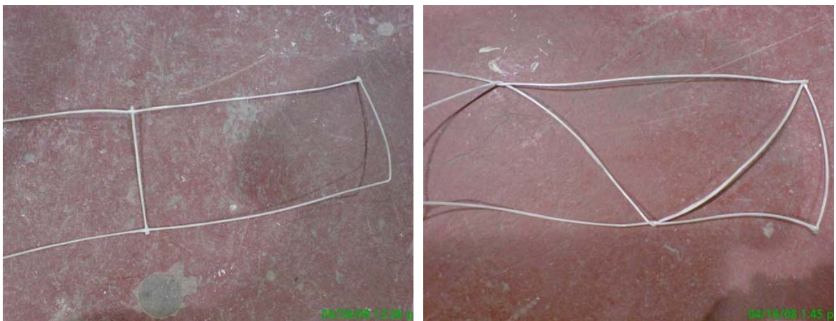
Figure 3.10: GFRP BJR (Ladder Shape) in Wall-G(L) (left) and (Truss Shape) in Wall-G(T) (right)
