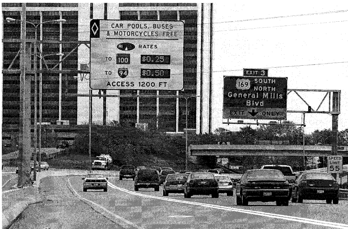
Figure 2.5 DMS at access point to HOT lane in Minneapolis – St. Paul (Image Courtesy of MnDOT)
