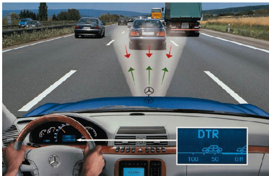
Figure 1.3: DISTRONIC Adaptive Cruise Control in a Mercedes-Benz [Mercedes-Benz, 2004].
