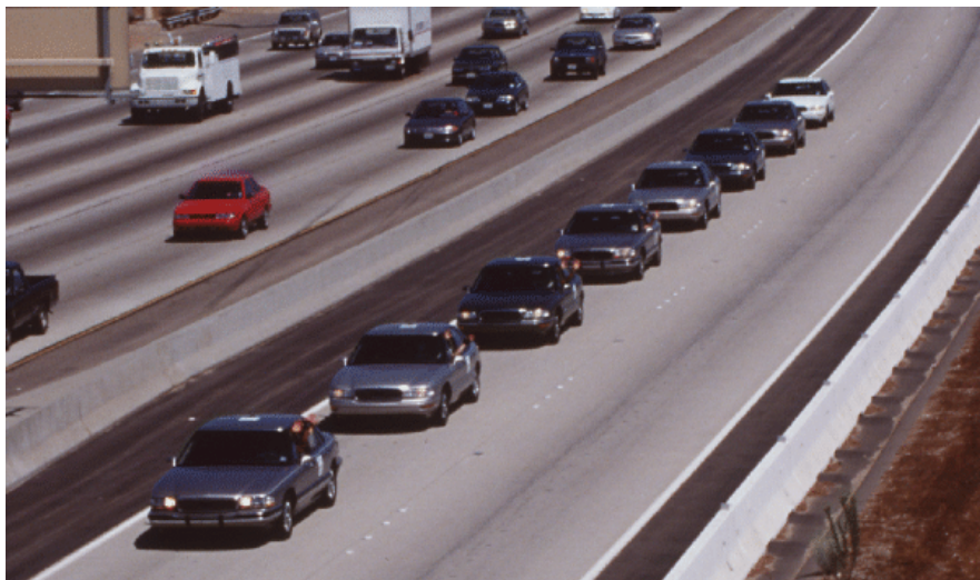
Figure 1.1: Platoon of automated vehicles on an Automated Highway System, developed by the PATH project [Hedrick et al., 1994].
