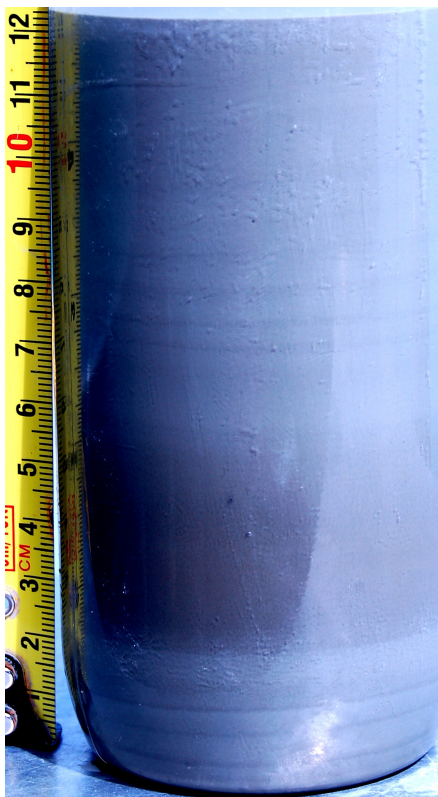
Figure H.1 Photograph of sediment trap immediately after removal from mooring C. Trap was deployed 0.5 m from the lake bottom from June 27 to July 12, 2007. For mooring location see Fig. 4.1.
