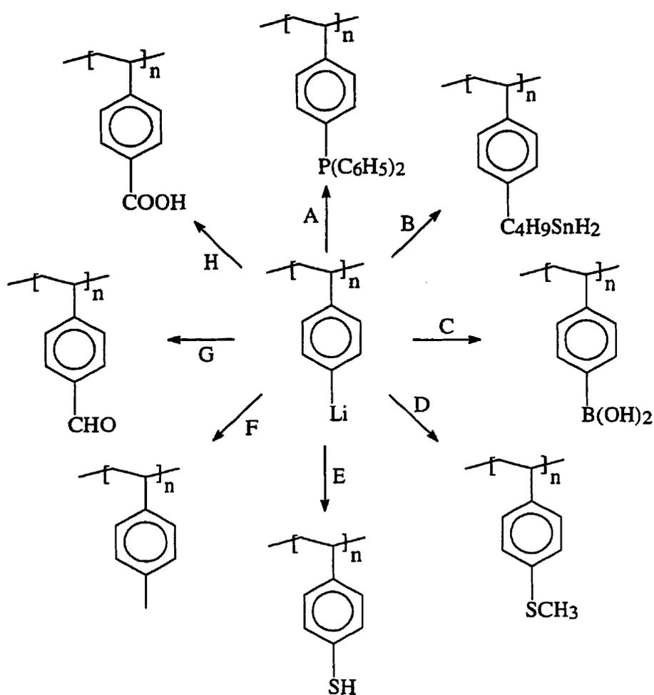
**Figure 1.9** Reaction of lithiated polystyrene
