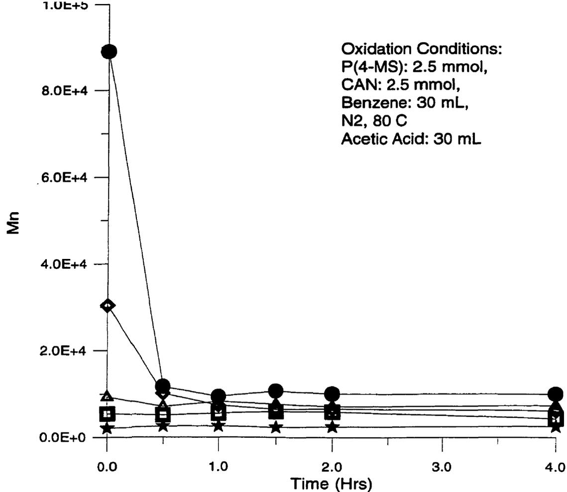
**Figure 4.3** The changes in Mn with time during the oxidation of P4MS
