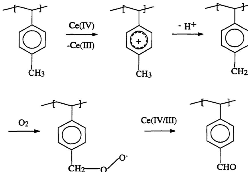
**Figure 2.4** Oxidation mechanism of poly(4-methylstyrene) by
