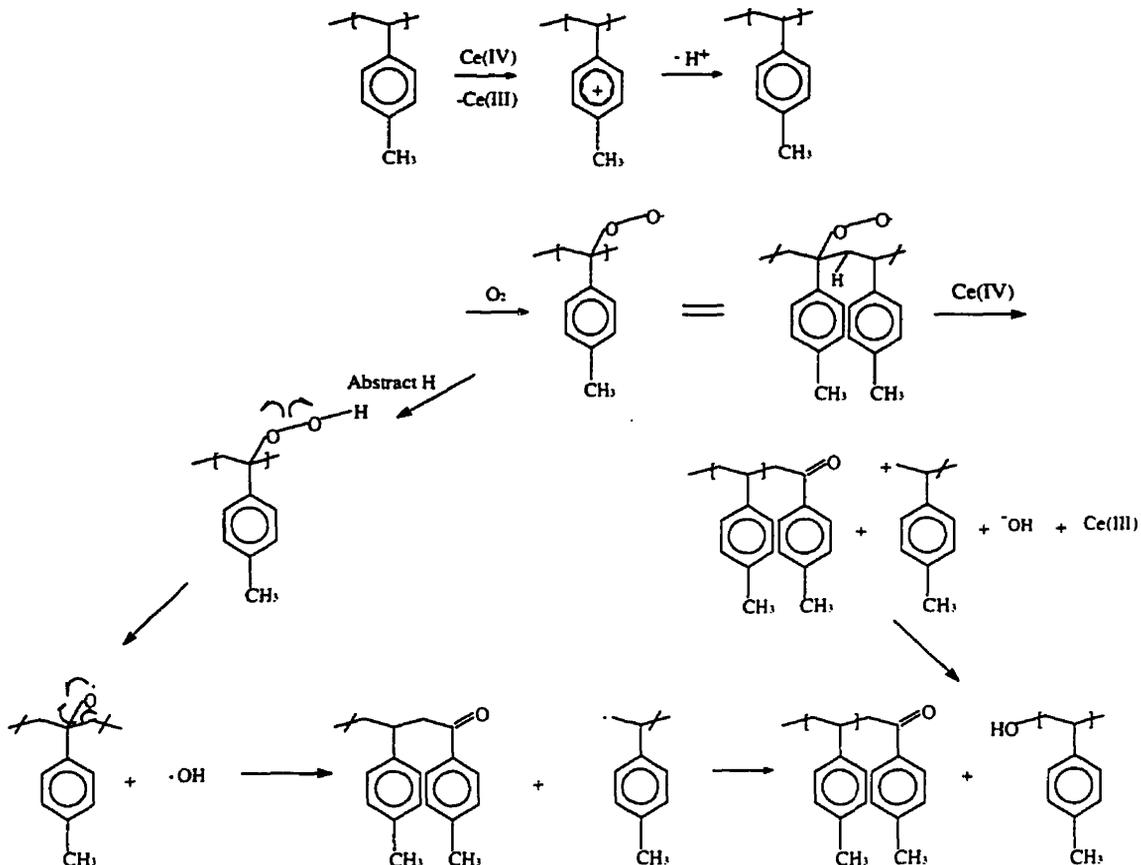
**Figure 4.2.** Degradation mechanism of poly(4-methylstyrene) by CAN/oxygen
