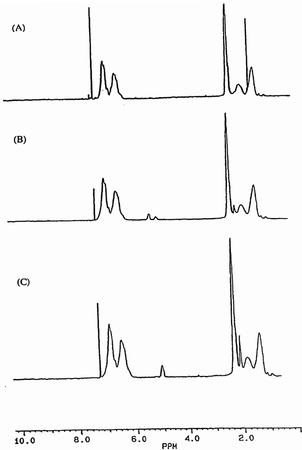
**Figure 2.1**  $^1\text{H}$  NMR spectrum. (A): Poly(4-methylstyrene), (B): after oxidation of poly(4-methylstyrene) by cerium ammonium nitrate, (C): after displacing the nitrate group.
