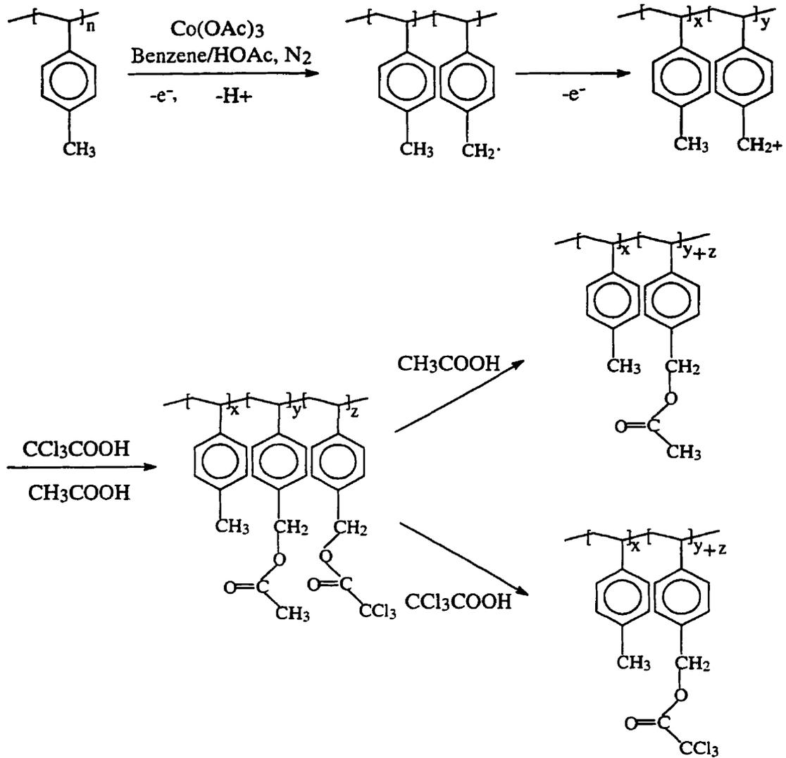
**Figure 3.5** Oxidation of poly(4-methylstyrene) by cobalt (III) acetate
