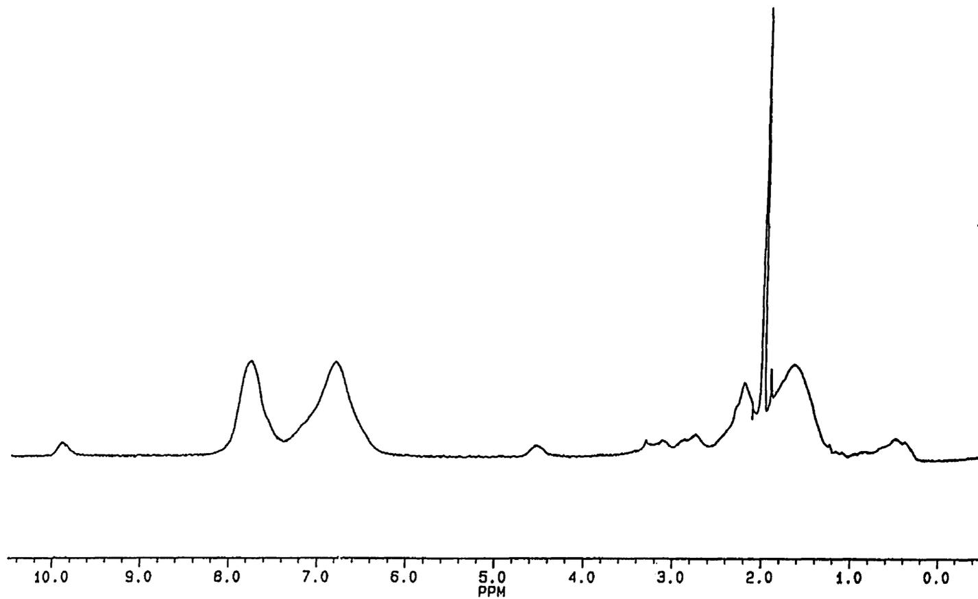
**Figure 5.14** <sup>1</sup>H NMR spectra of copolymers of 4-methylstyrene and methyl methacrylate with 10:1 feed ratio after Co(II) oxidation
