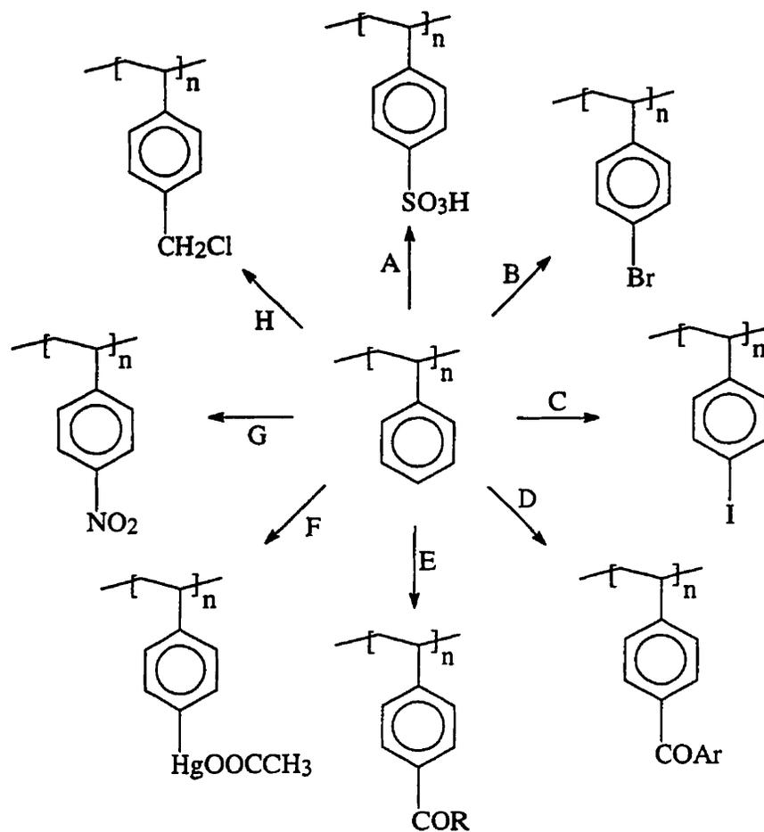
**Figure 1.7** Electrophilic aromatic substitution reactions of polystyrene
