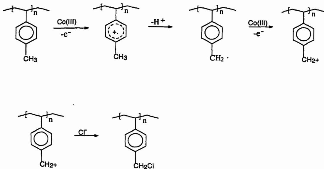
**Figure 3.7** Mechanism of oxidation of poly(4-methylstyrene) by Cobalt(III) acetate/lithium chloride system
