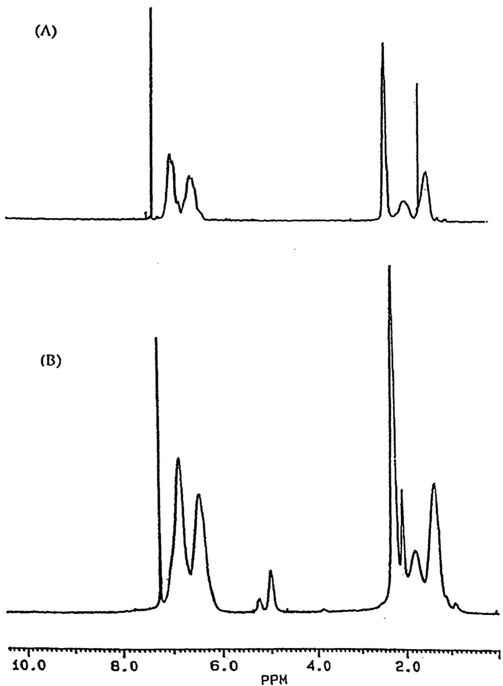
**Figure 3.1**  $^1\text{H}$  NMR spectrum. (A): Poly(4-methylstyrene), (B): after oxidation of poly(4-methylstyrene) by cobalt(III) acetate/trichloroacetic acid.
