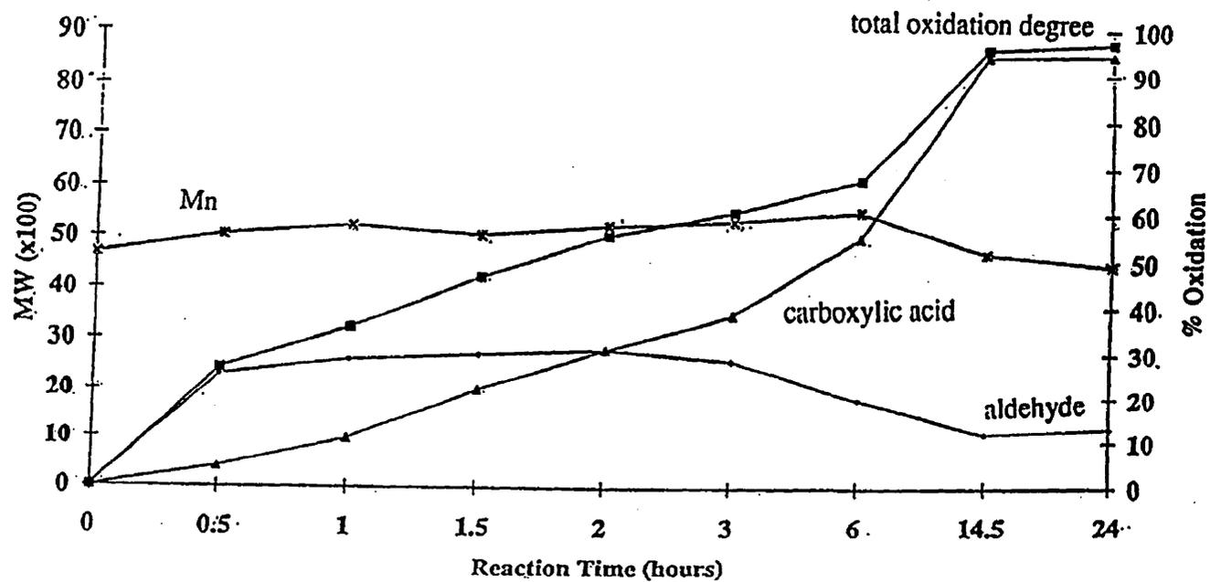
Figure 5.2 Oxidation of poly(4-methylstyrene-co- $\alpha$ -methylstyrene)
