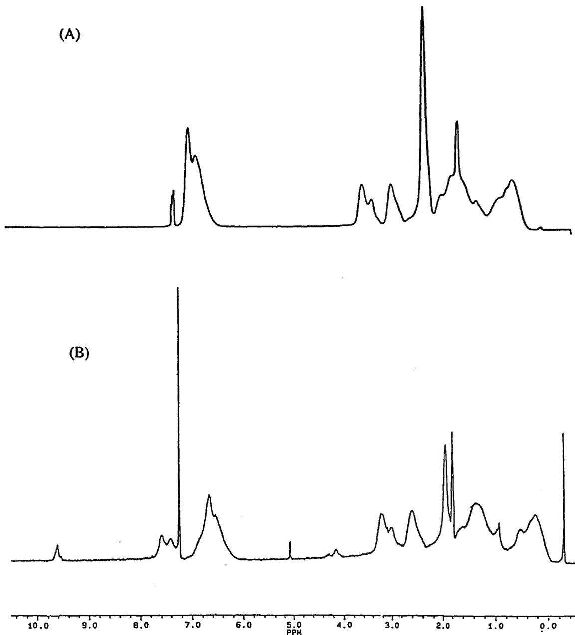
**Figure 5.9**  $^1\text{H}$  NMR spectra of copolymer of 4-methylstyrene and methyl methacrylate after Co(II) oxidation: (A) Copolymer of 4-methylstyrene and methyl methacrylate. (B) Oxidized copolymer (containing 17.7 % of aldehyde and 29.5 % of carboxylic acid groups).
