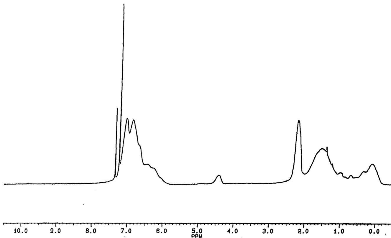
Figure 5.3  $^1\text{H}$  NMR spectrum of copolymer of 4-methylstyrene and  $\alpha$ -methylstyrene (containing 13.0 % of chloromethyl group)
