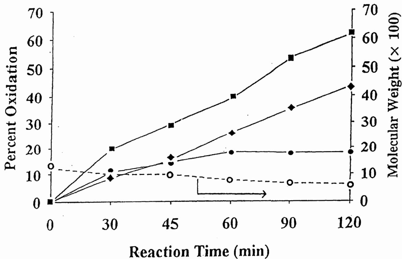
**Figure 5.1** Oxidation rate and backbone cleavage in heptane/acetic acid. Reaction conditions: 3 g poly(4-methylstyrene) in 150 mL acetic acid/heptane 1:1, 10 mol% catalyst, 80°C, oxygen flow rate: 400 mL min<sup>-1</sup>.
