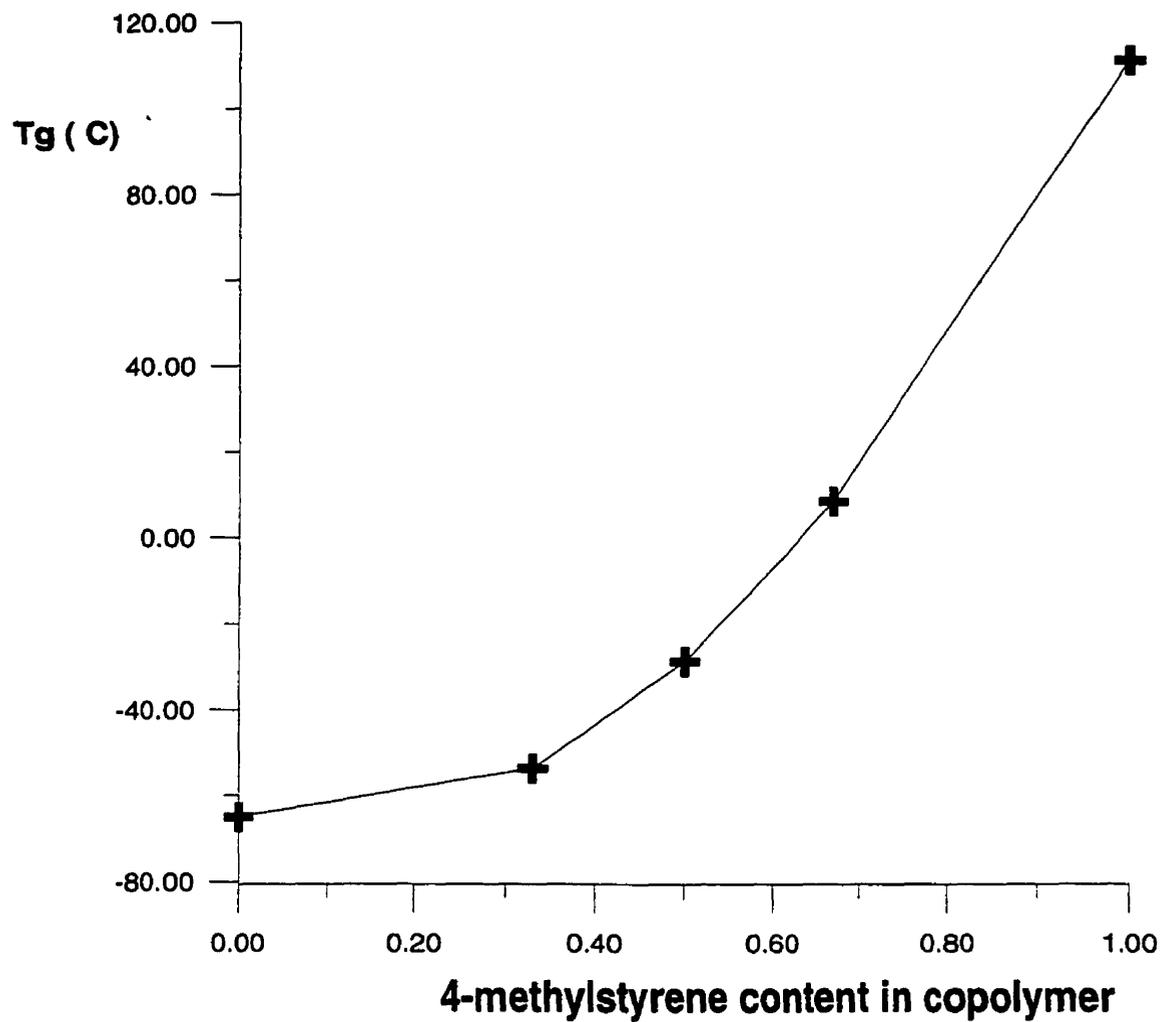
**Figure 6.7** Tg and monomer feed ratio for the copolymer of 4MS/DMA.
