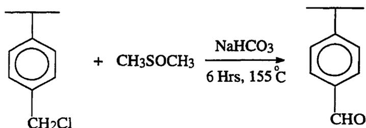
To test the presence of chlorine in the oxidized polymer, the same oxidation with DMSO was carried out. The  $^1\text{H}$  NMR spectrum (Figure 3.4) of the reaction product showed the presence of the benzaldehyde proton (9.9 ppm), and ortho protons of the aldehyde group of the benzene ring (7.48 ppm), but no chloromethyl protons. There was also no spectral or chemical evidence of functional groups other than aldehyde. In addition, some crosslinked polymer was obtained.<sup>27</sup>
