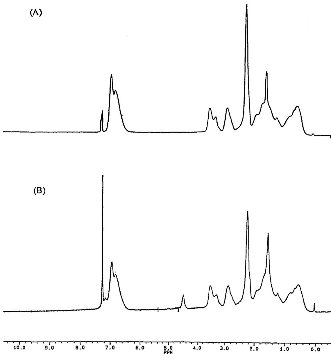
**Figure 5.10** <sup>1</sup>H NMR spectra of copolymer of 4-methylstyrene and methyl methacrylate after Co(III) oxidation: (A) Copolymer of 4-methylstyrene and methyl methacrylate. (B) Oxidized copolymer (containing 24.2 % of chloromethyl groups).
