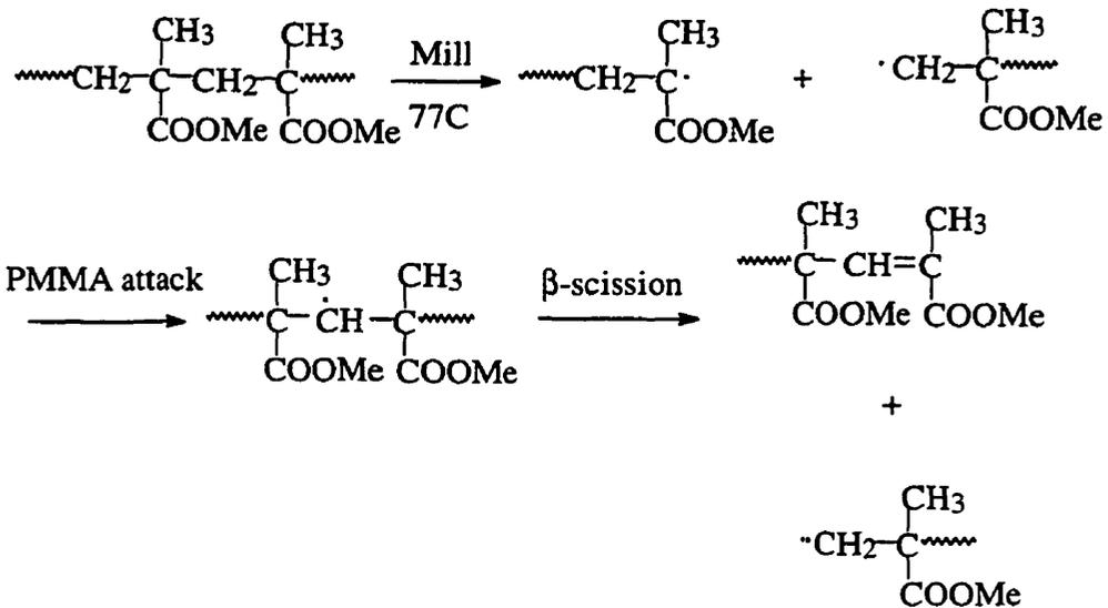
During mechanical degradation, the molecular weight of a polymer decreases with time as illustrated in Figure 4.1:<sup>32</sup>
