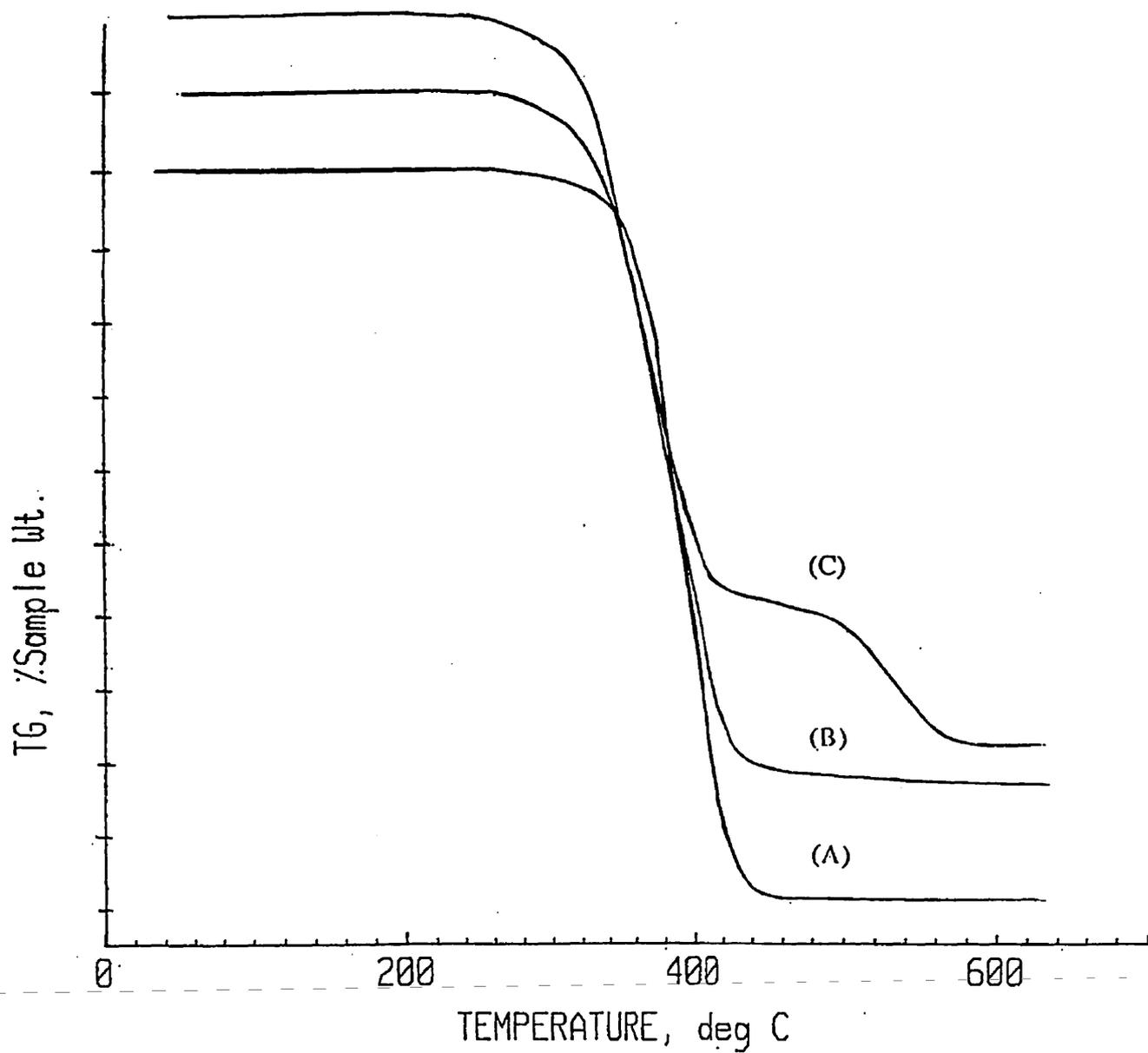
**Figure 6.4** Thermograms of poly(4-methylstyrene) in nitrogen (A), a-35 (containing 23.7% of acetoxymethyl group) in nitrogen (B) and in air (C). Each plot begins at 100% on the mass axis, with each division representing a 10% mass loss
