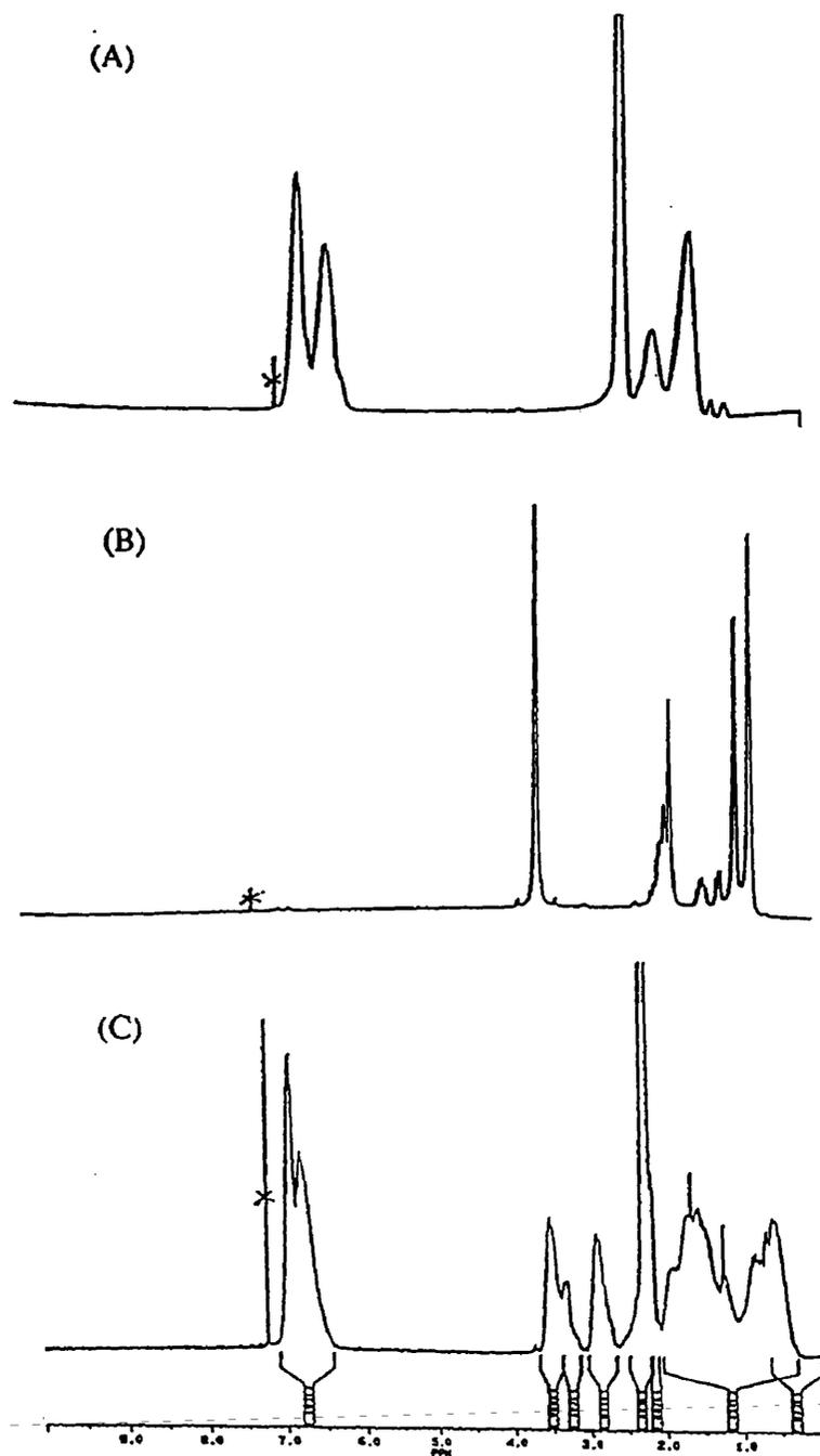
Figure 5.8 <sup>1</sup>H NMR spectra of poly(4-methylstyrene) (A), poly(methyl methacrylate) (B), and poly(4-methylstyrene-co-methyl methacrylate) (1:1) (C).
