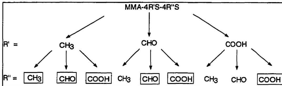
**Figure 5.12** Environments after oxidation for 1:2 copolymer, Poly(methylmethacrylate-*co*-4-methylstyrene)
