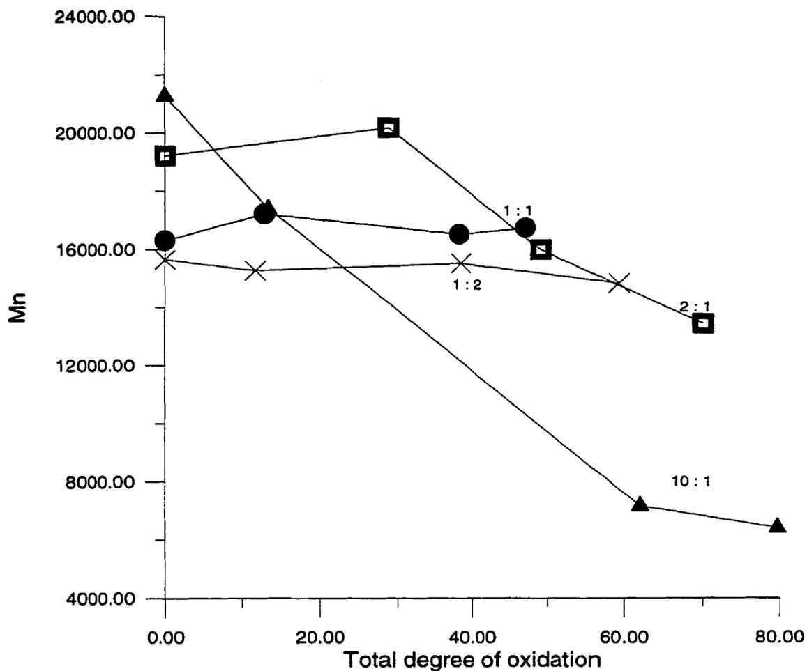
**Figure 5.15** Relationship of molecular weight and oxidation yield for copolymers of 4-methylstyrene and methyl methacrylate ( data from Table 5.10, 5.11, 5.12 and 5.13)
