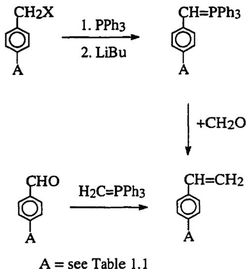
**Figure 1.4** Synthesis of styrene derivatives via Wittig reaction
