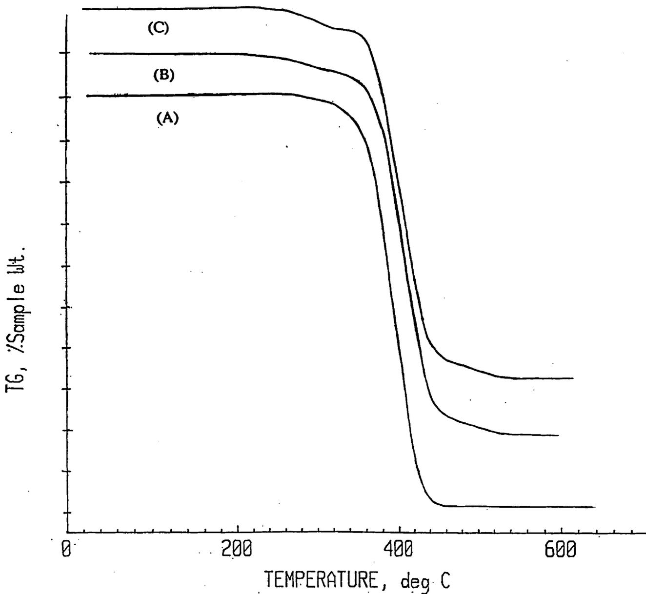
**Figure 6.2** Thermograms in nitrogen of poly(4-methylstyrene) (A), sample 10 (containing 12.5% of chloromethyl group) (B), and sample 18 (containing 21% of chloromethyl group) (C). Each plot begins at 100% on the mass axis, with each division representing a 10% mass loss
