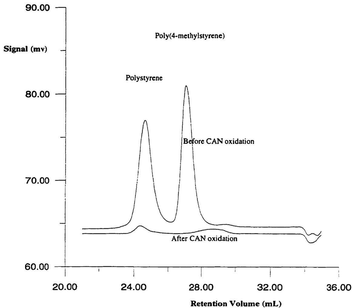
**Figure 4.4** GPC Overlays of the mixture of poly(4-methylstyrene) and polystyrene before and after oxidation
