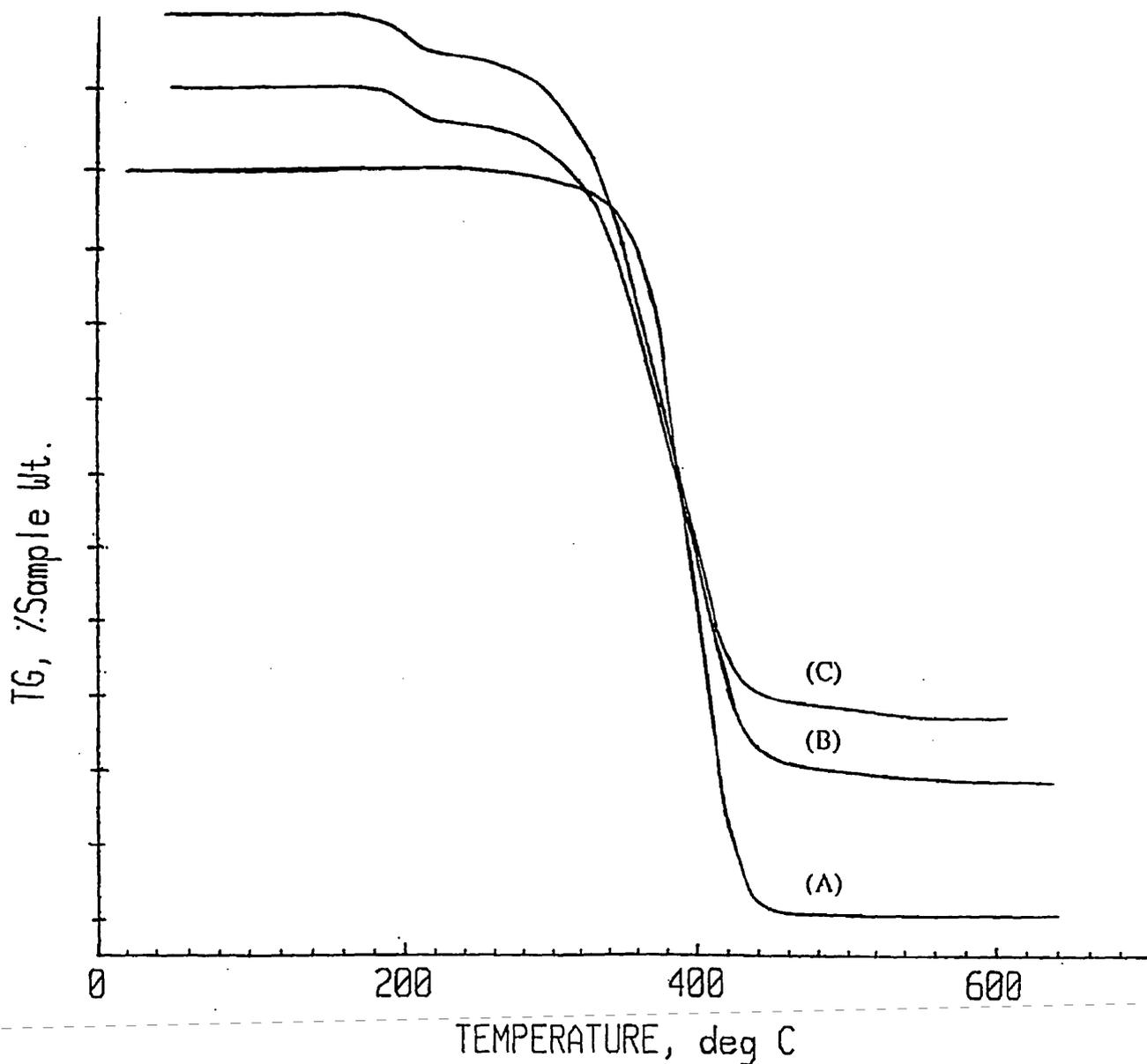
**Figure 6.5** Thermograms of poly(4-methylstyrene) (A), a-25 (B), and a-11 (C) (containing 23.6% and 45.2% total oxidation degree respectively) under nitrogen. Each plot begins at 100% on the mass axis, with each division representing a 10% mass loss division representing a 10% mass loss.
