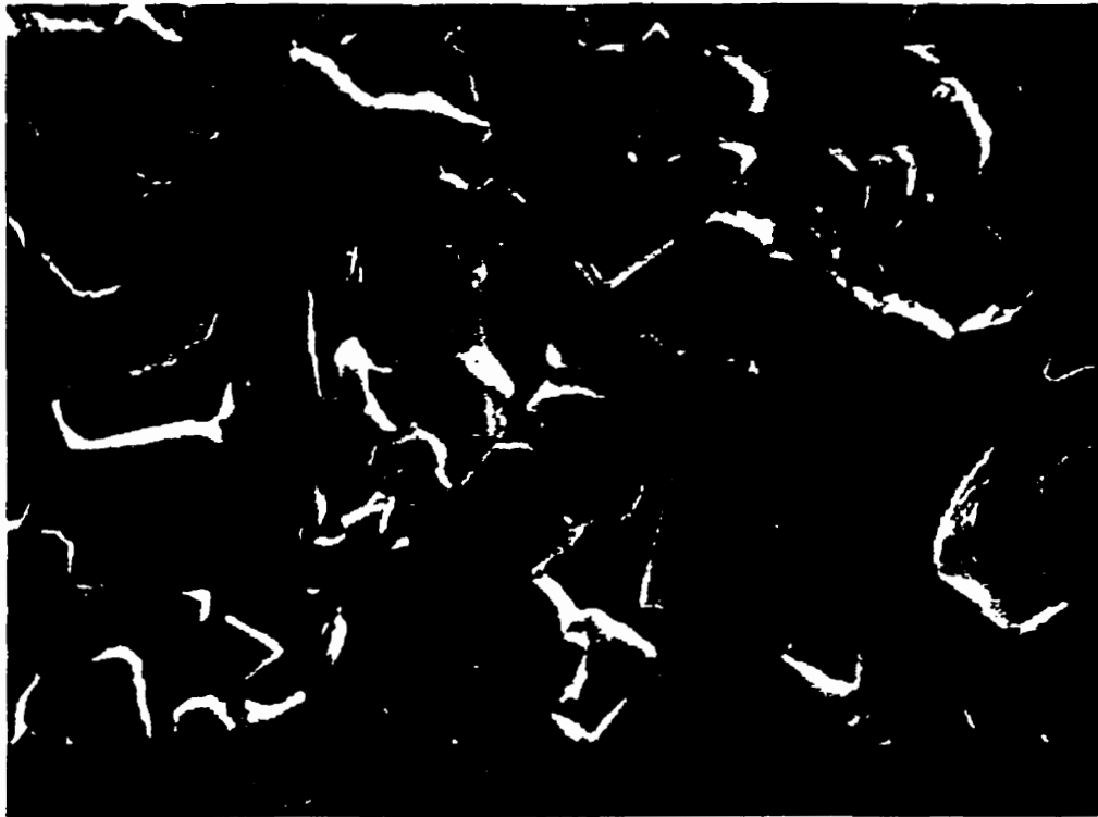
Figure 4-32. Micrograph of polished CAS surface after devitrification.
