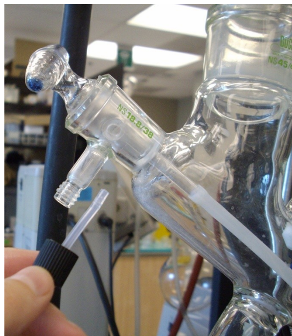
Figure 3.8 Close-up of rotary evaporator stopcock arrangement
