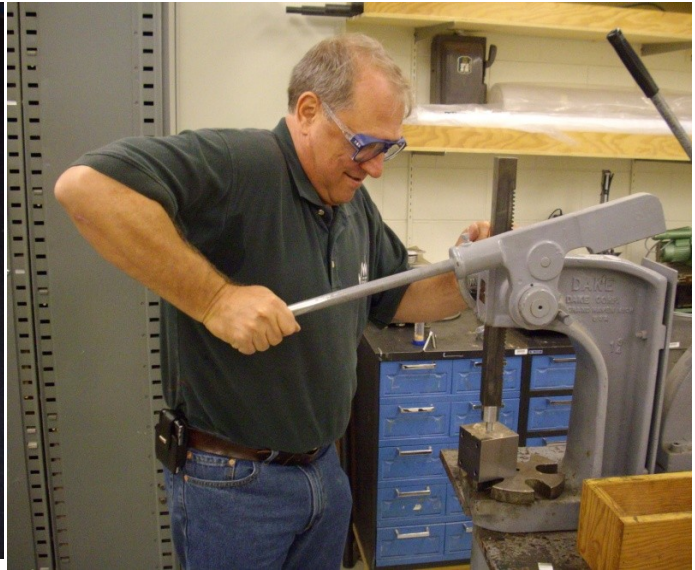
Figure 3.10b High pressure press arrangement where plunger compresses sample in a gamma tube housed in the steel die
