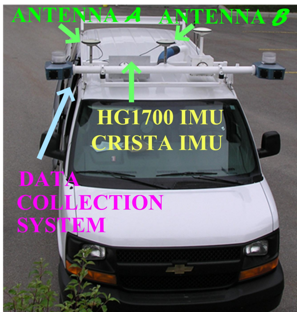
Figure 3.1 Vehicle Test Setup
