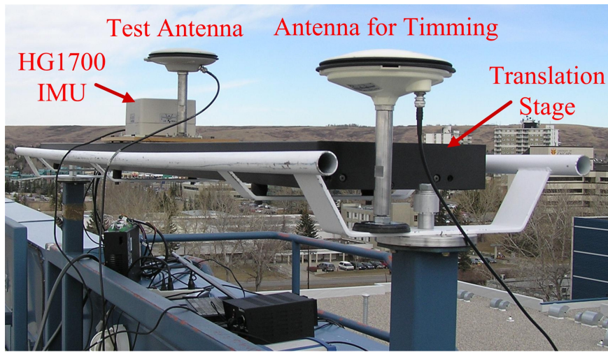
Figure 4.5 Translation Stage Test Setup
