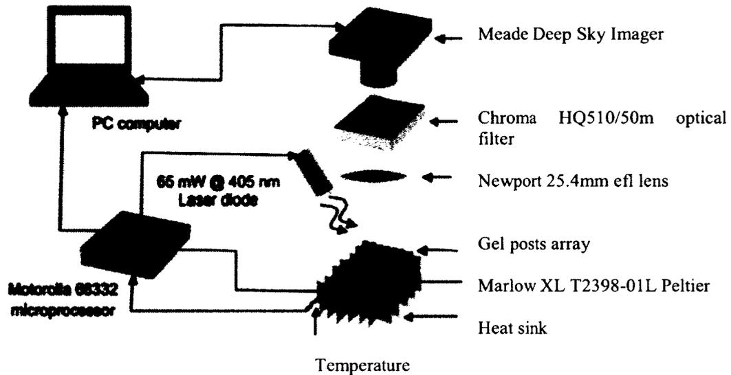
The printed gel posts on the coverslip are placed in the Viriloc for thermal cycling, and the raw fluorescence during the PCR and MCA can be captured by the camera and sent to the computer. Once the PCR/MCA is finished, the analysis is done using software ImageJ.xla [83].
