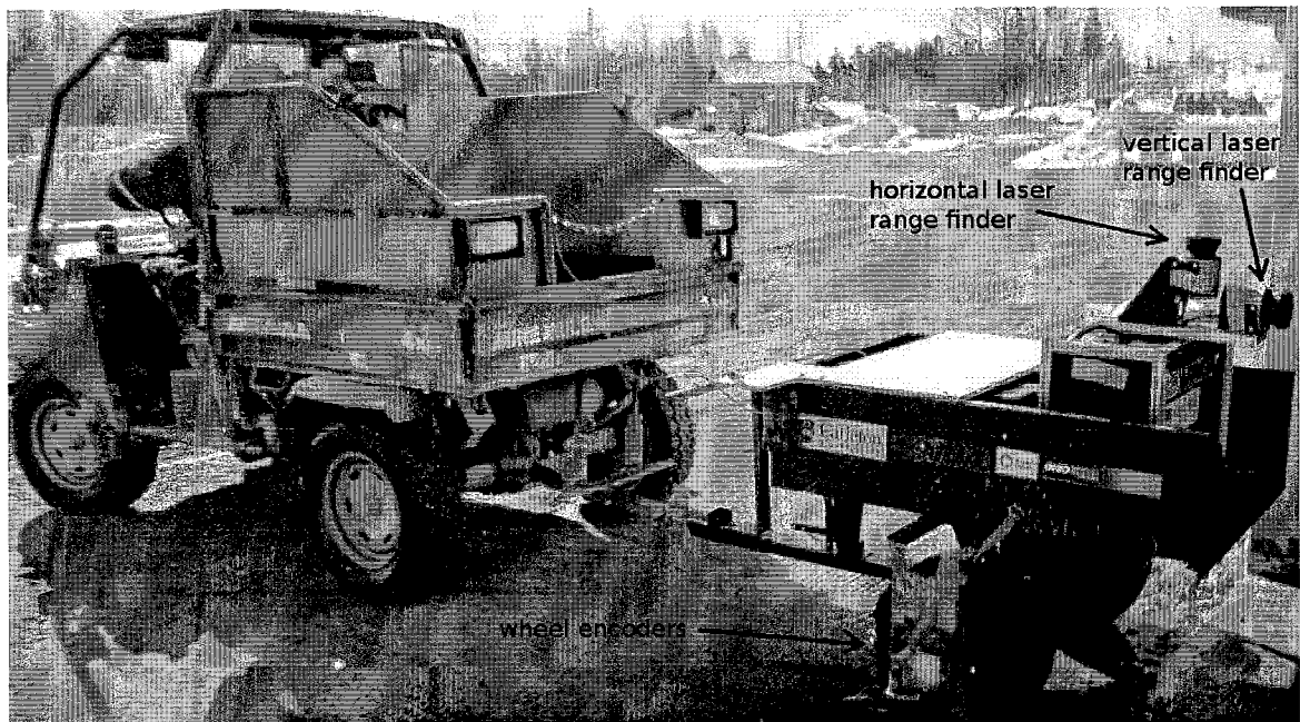
Figure 4.2: Utility trailer with sensors attached to MineMule at CANMET Experimental Mine.
