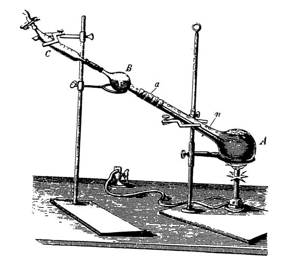
Figure 3. The apparatus of Lothar Meyer for measuring blood gases. From L. Meyer, Die Gases des Blutes (1857) Plate II. For description see p. 73 opposite
