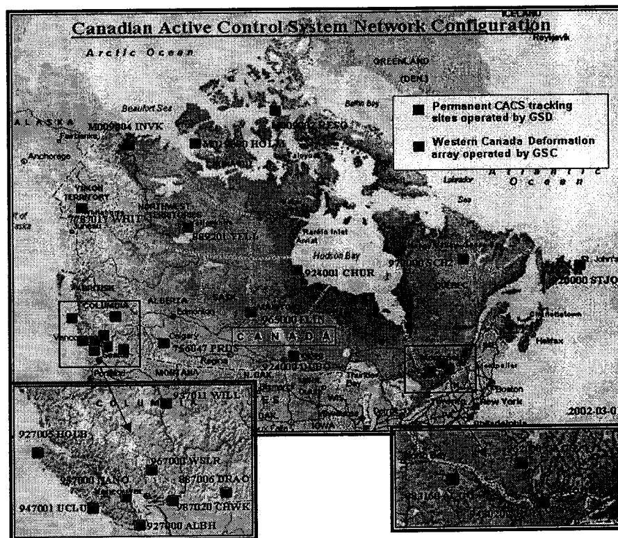
Figure 3.2 Canada-wide CACS Network [http://www.geod.nrcan.gc.ca/index_e/products_e/activeNetwork_e/acp_e.html]
