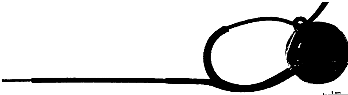
Figure 2.2 Model RI-2B radio transmitter and adjustable elastic necklace (Holohil Systems Ltd., Ontario, Canada)
