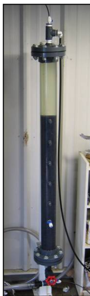
Figure 4-9 - Manganese dioxide pilot column used in Experiment II
