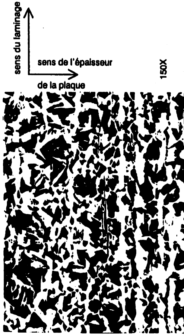
Figure II.1: Microstructure de l'acier SA-516-70
