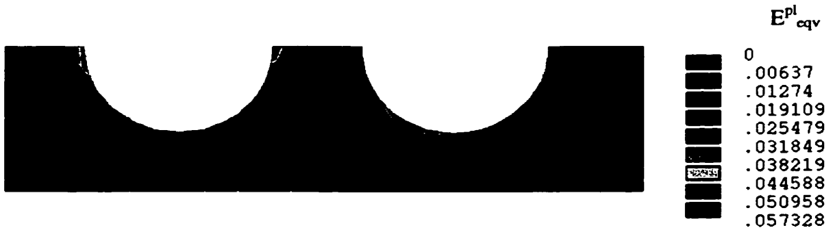
Fig. 5-43 Two dimensional equivalent plastic strain for cold expanded hole.
